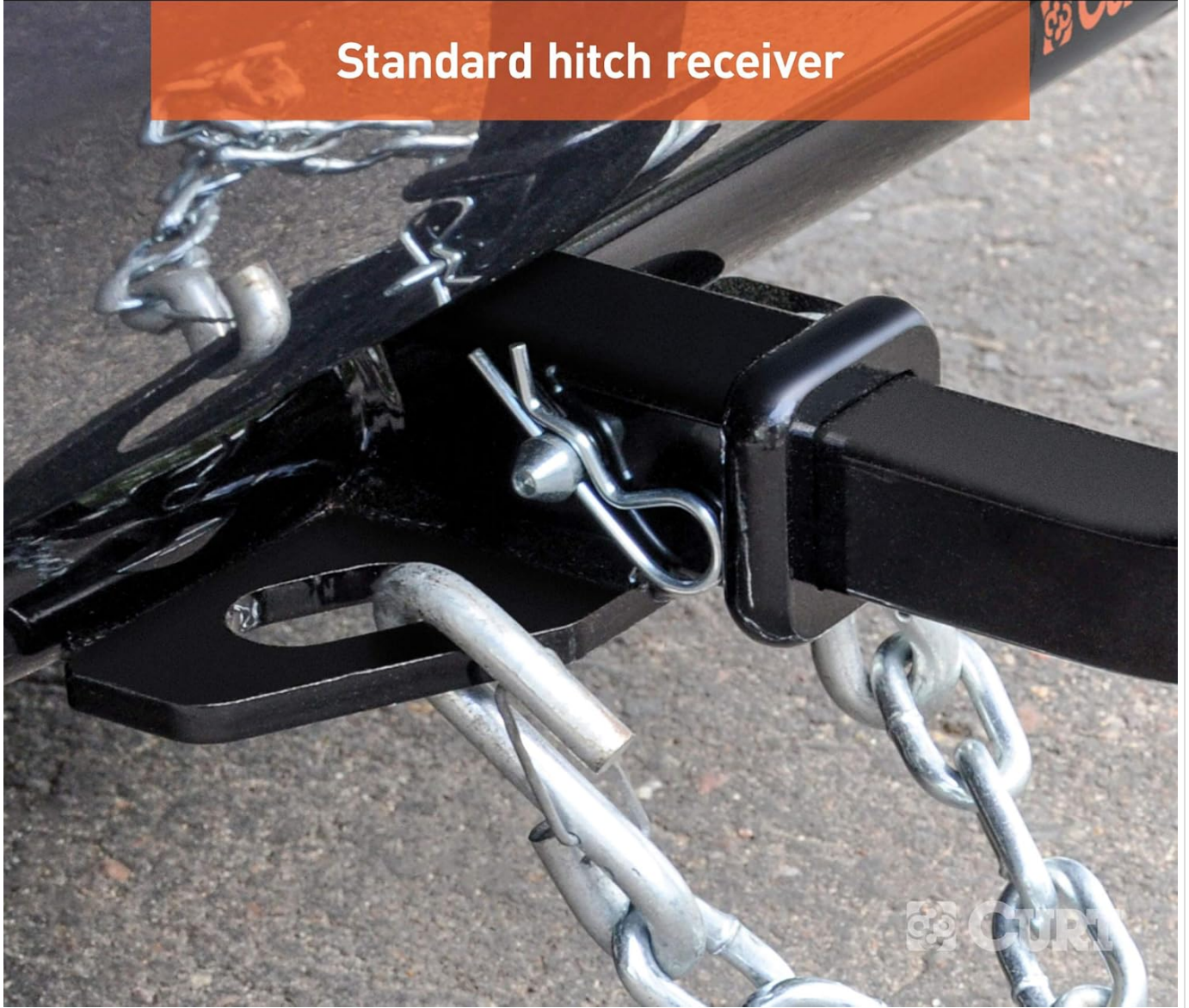
Image: A close-up view of the standard hitch receiver with a ball mount inserted and safety chains properly connected to the chain loops.
