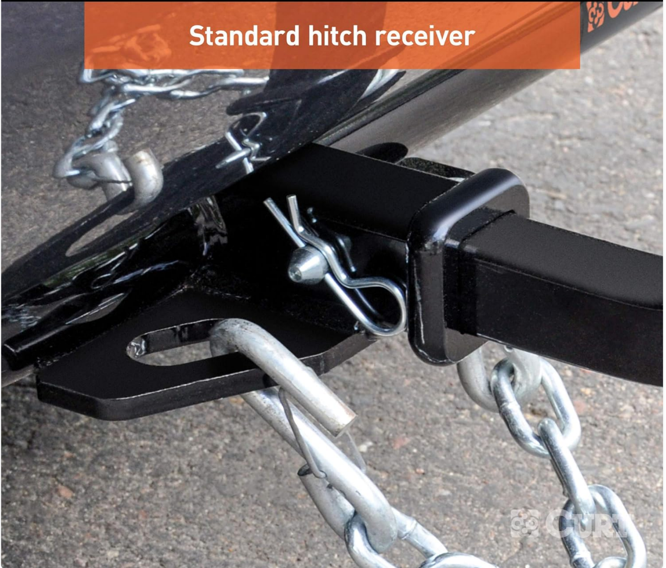
Image: A close-up view of a standard hitch receiver, demonstrating how safety chains are connected.
