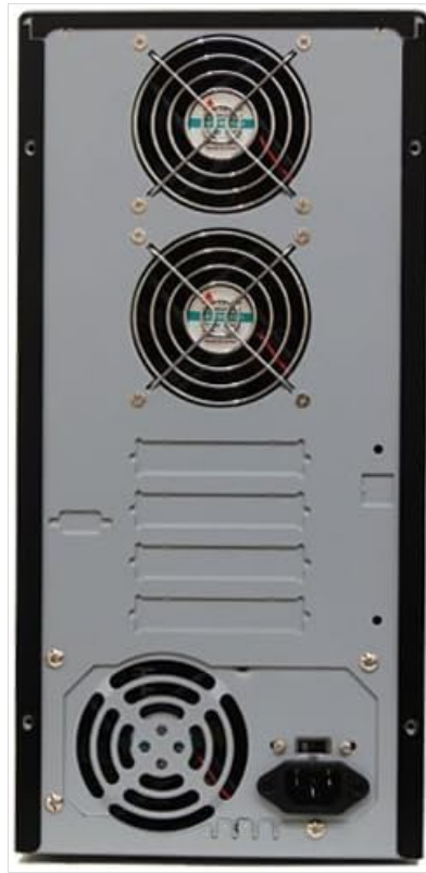
Figure 4.3: Rear Panel Components (Power input and cooling fans)
