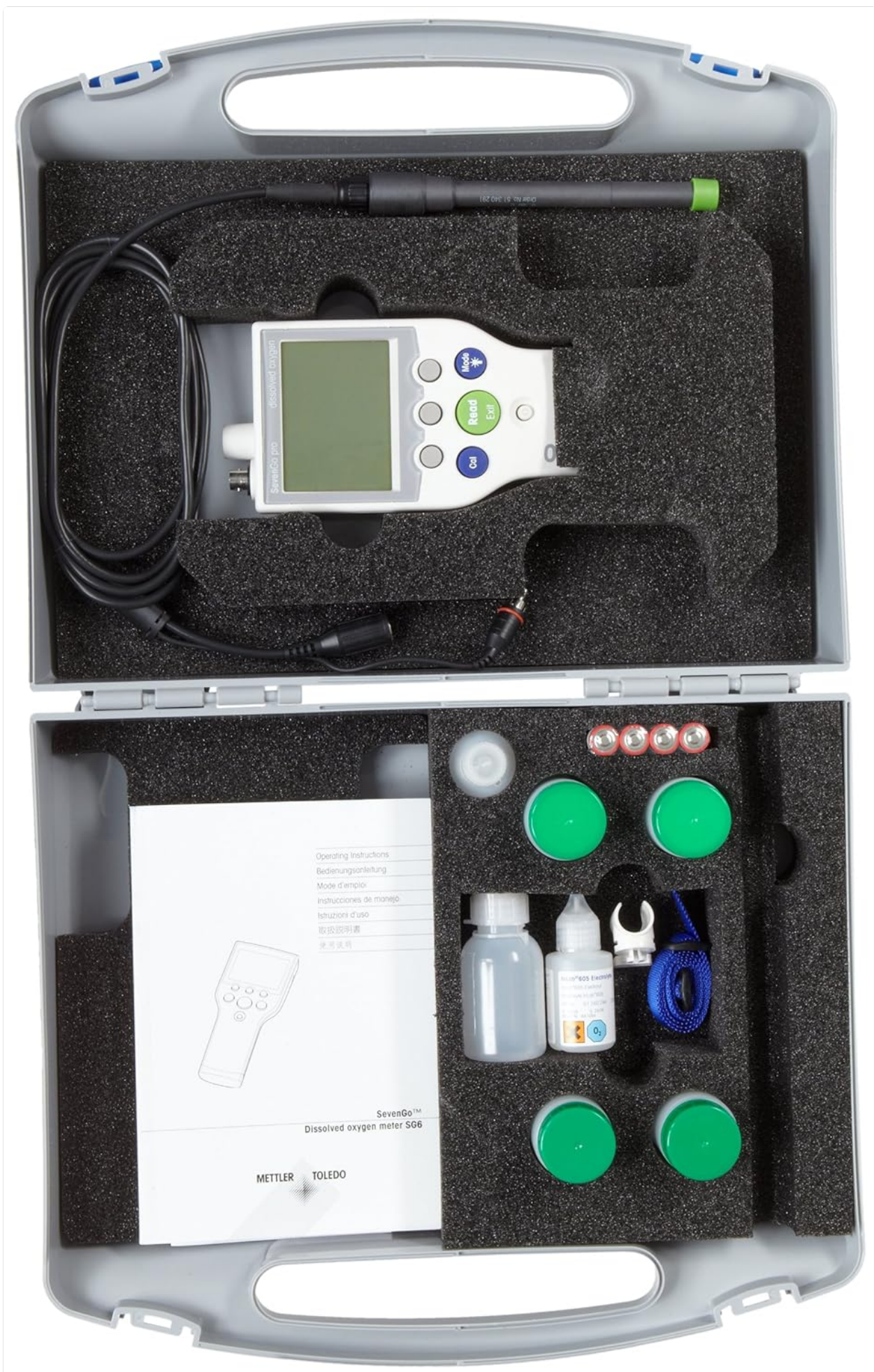
Figure 3.1: Contents of the Mettler Toledo SevenGo Pro Field Kit, including the meter, electrode, and various accessories within its protective carrying case.
