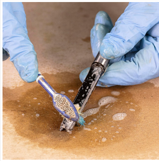
Image: Scrubbing the router bit with a toothbrush to remove stubborn residue.
