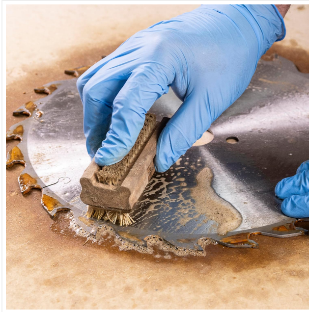
Image: Scrubbing the saw blade with a brush to remove loosened debris.
