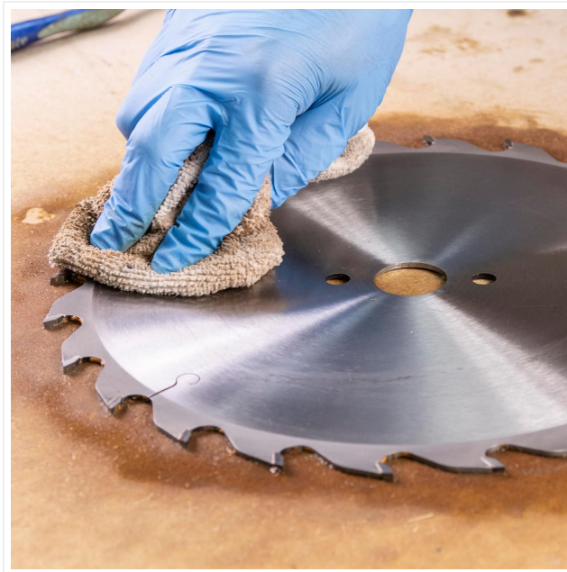
Image: Wiping the saw blade clean after scrubbing, revealing a polished surface.
