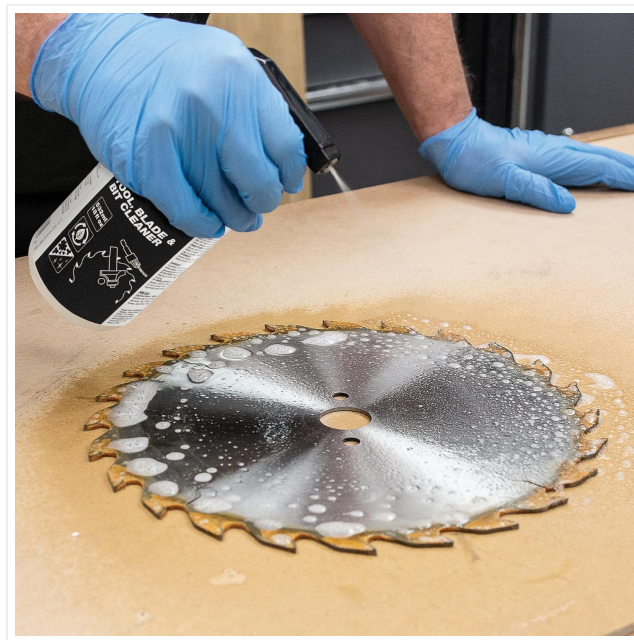
Image: Applying the cleaner to a saw blade to loosen resin and grime.
