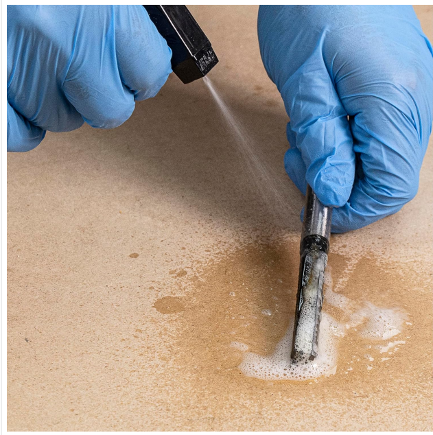
Image: Applying the cleaner to a router bit to dissolve accumulated resin.
