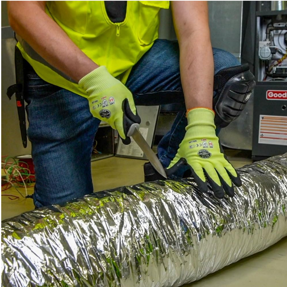
Figure 4: A user demonstrating the application of the Klein Tools DK06 Duct Knife for cutting flexible duct material.
