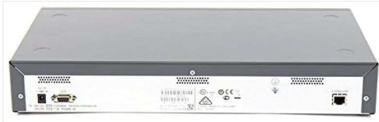
Figure 2.3: Rear view of the Avaya IPO IP500 EXP MOD-PHONE 30 module, displaying the power input, serial port, and an Ethernet port.
