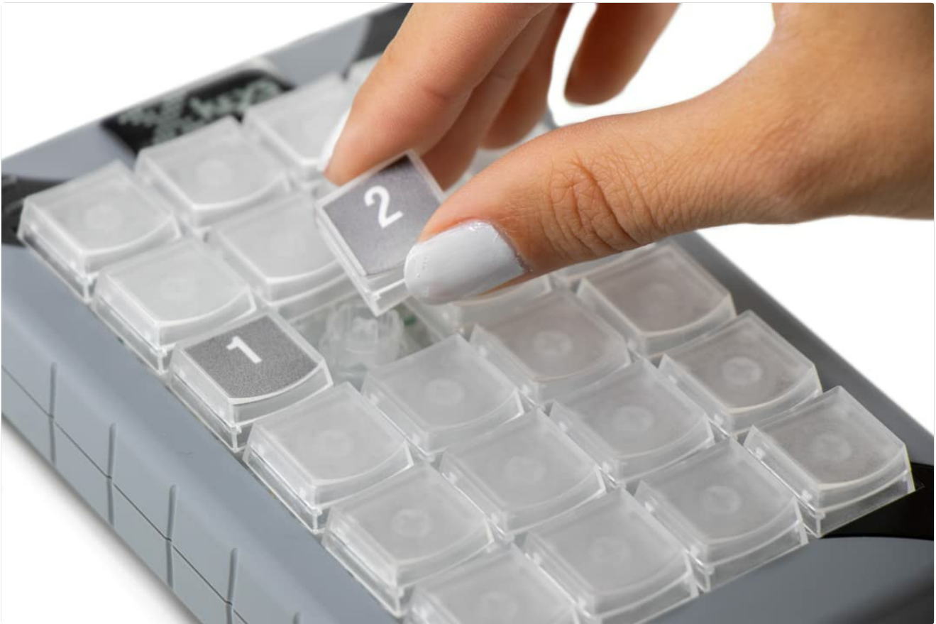
Figure 6: Demonstrating how to place a keycap.
