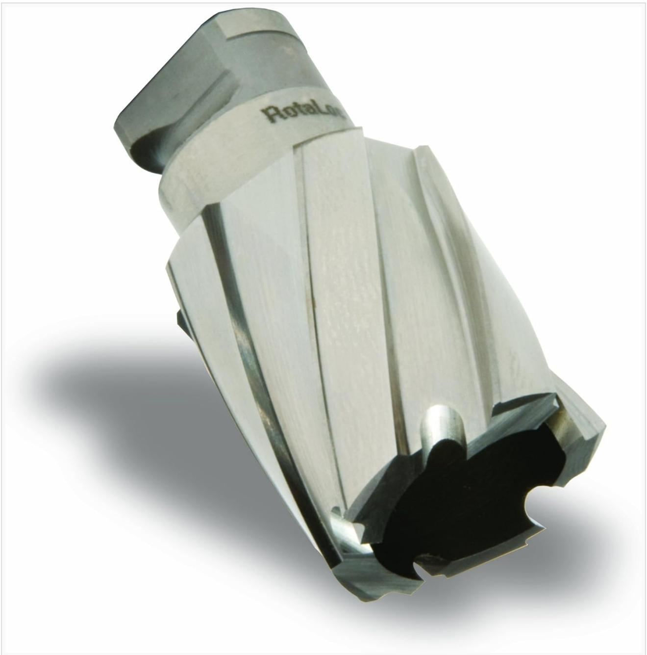
Image: The Hougén 17128 RotaLoc Annular Cutter, showcasing its bayonet-style shank and cutting teeth. This image illustrates the design of the cutter, highlighting its M42 high-speed steel construction and stack cut geometry.
