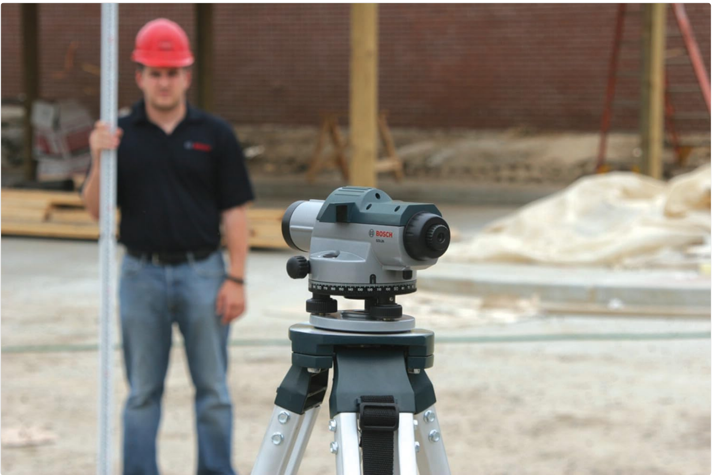
Figure 6: The BOSCH GOL26 optical level positioned on a tripod, with a person holding a leveling rod in the background, illustrating a typical measurement scenario.
