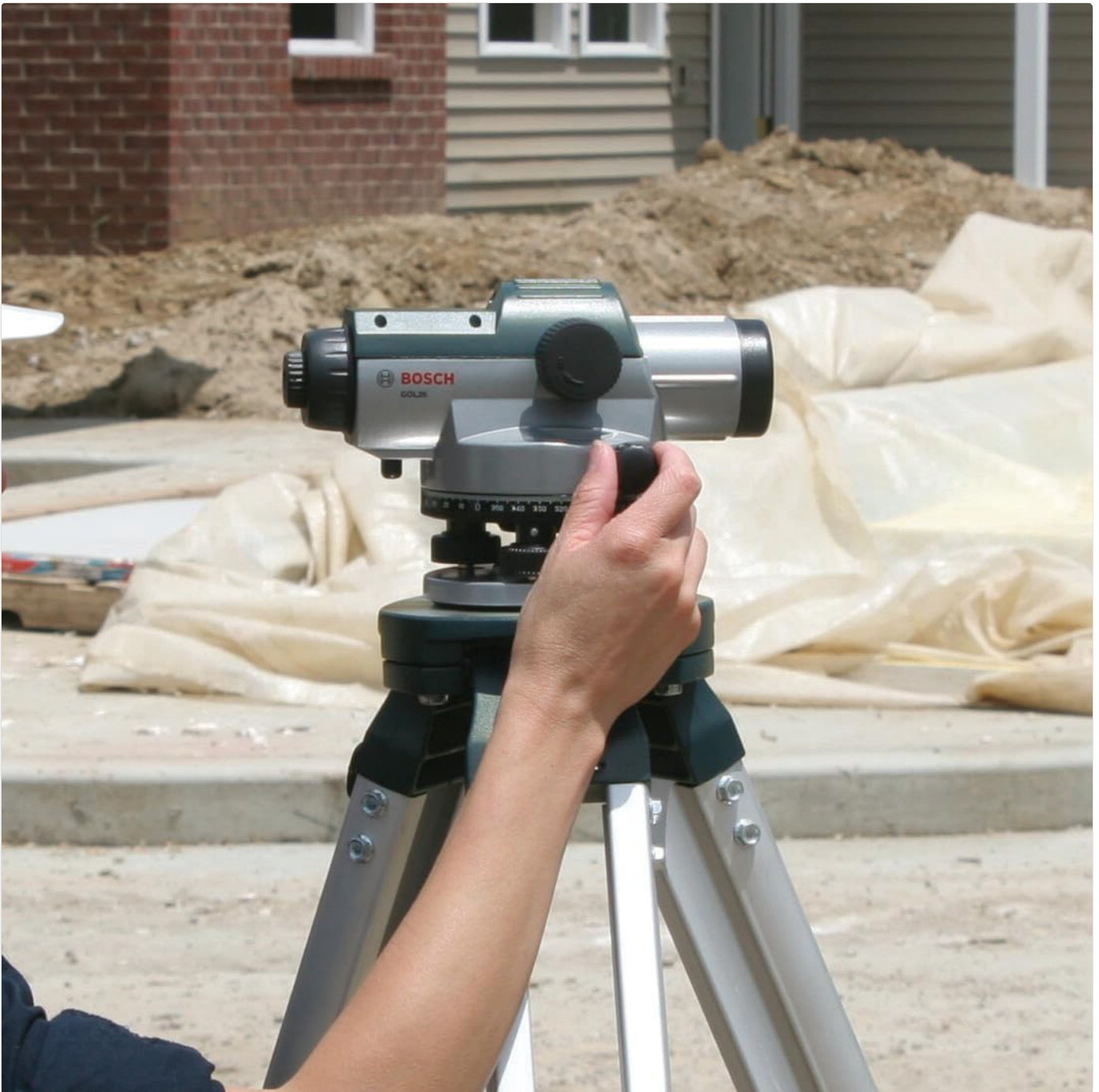
Figure 4: A close-up view of a hand making fine adjustments to the leveling screws on the optical level, ensuring precise calibration.
