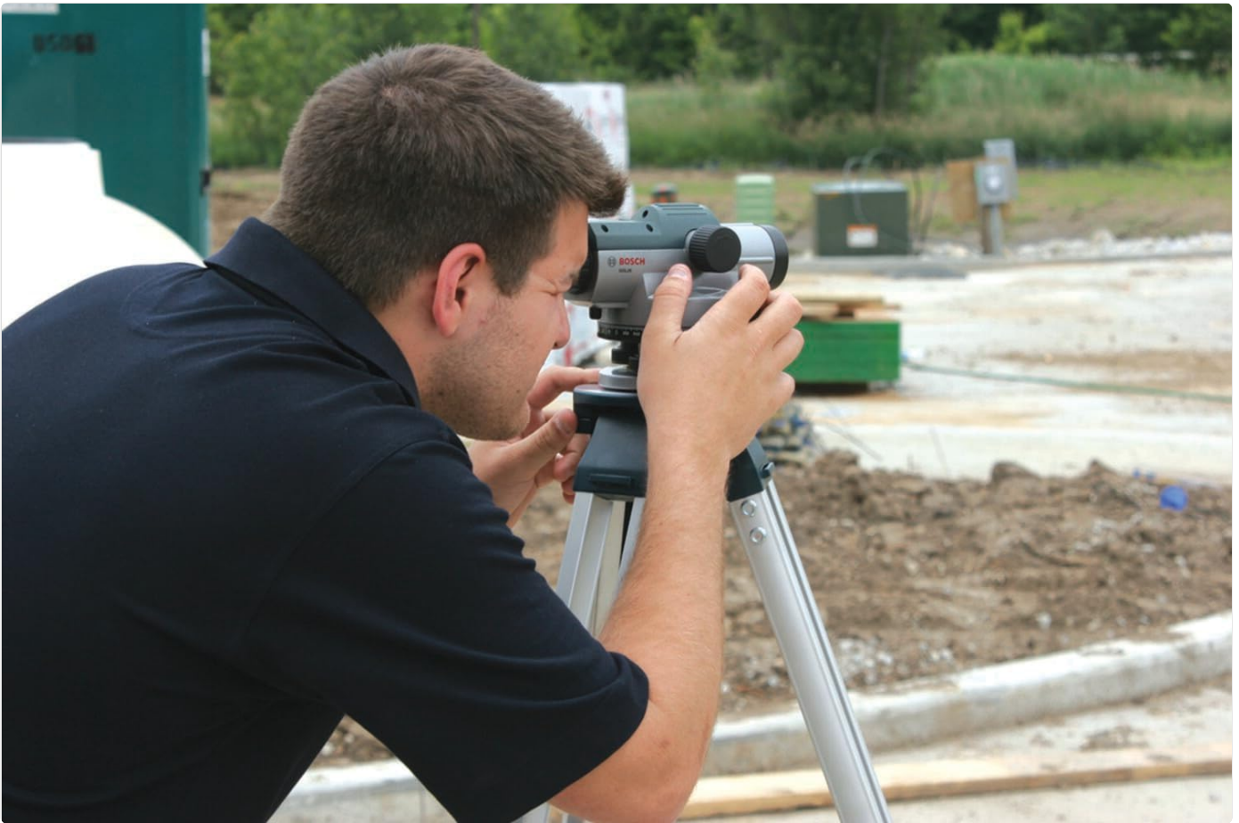
Figure 5: A user looking through the eyepiece of the BOSCH GOL26 optical level, demonstrating the process of taking a measurement.
