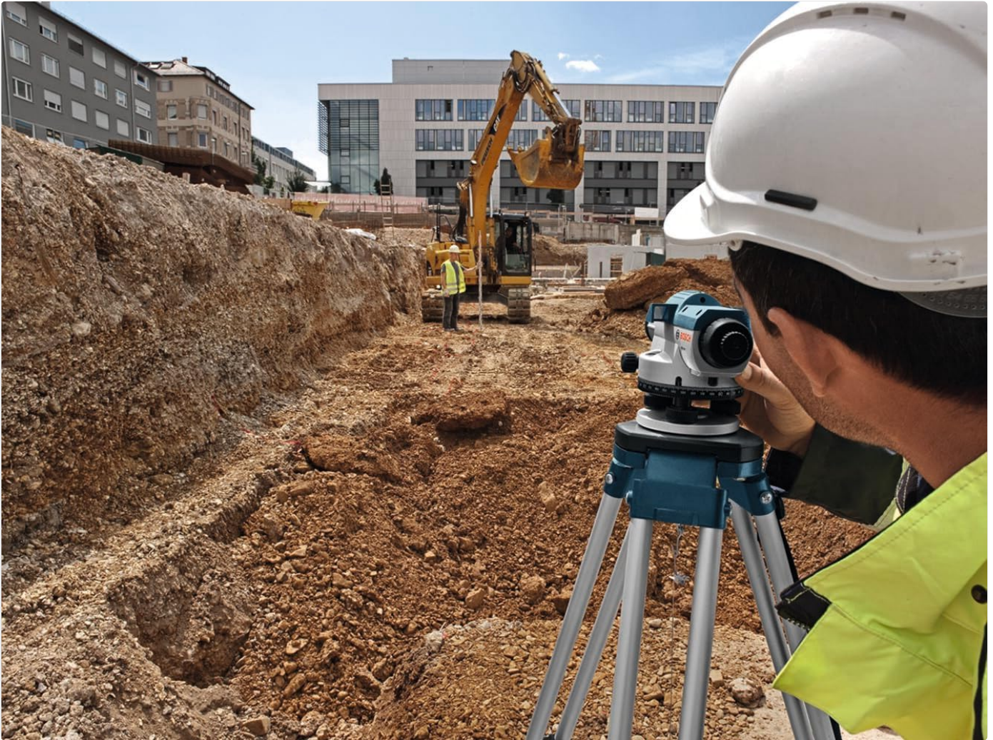
Figure 3: A user setting up the BOSCH GOL26 optical level on a tripod at a construction site, demonstrating typical field use.
