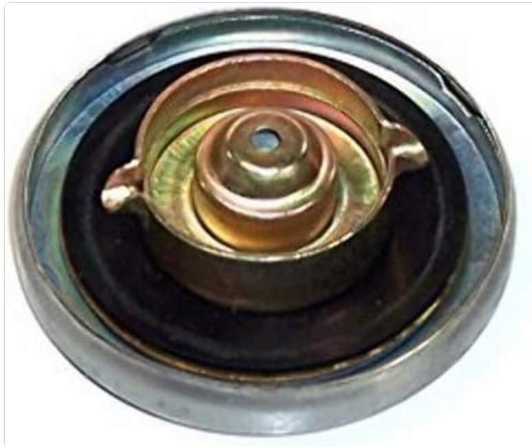
Figure 2: Underside view of the gas cap, illustrating the twist-on mechanism and seal.
