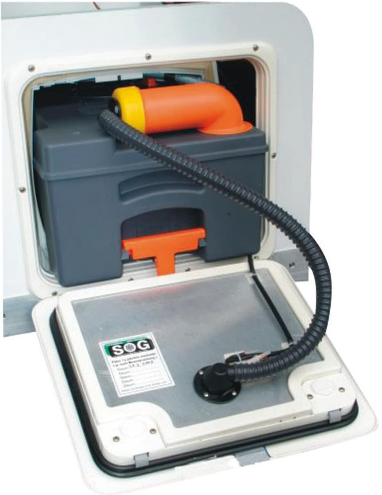
Figure 2: View of the toilet cassette compartment with existing ventilation setup.
