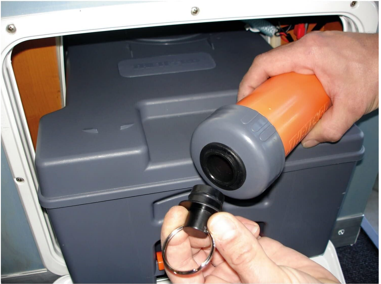
Figure 3: Preparing the connection point on the toilet cassette.
