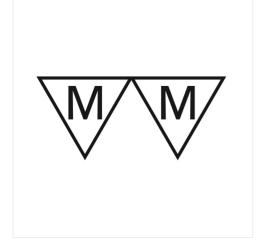
Image: The 'MM' symbol, indicating that the transformer is suitable for mounting on normally flammable surfaces.
