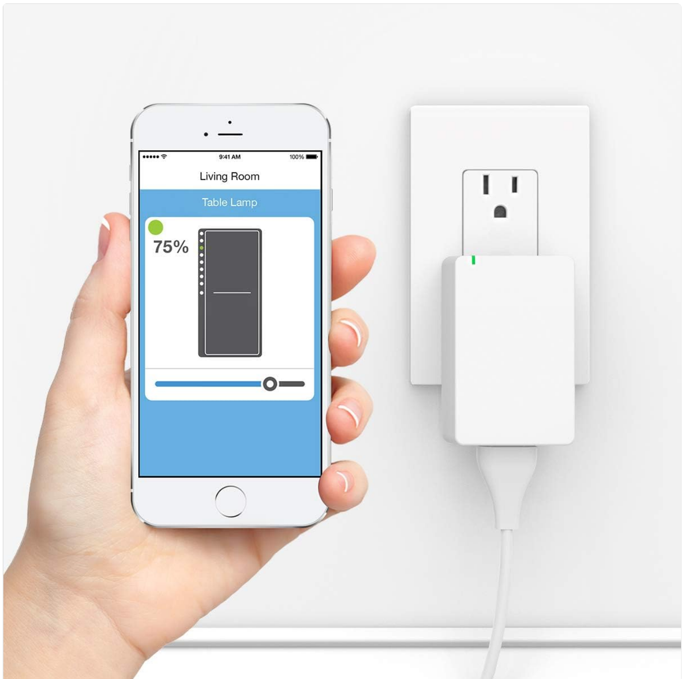
Figure 5: Smartphone control via the Insteon app.
