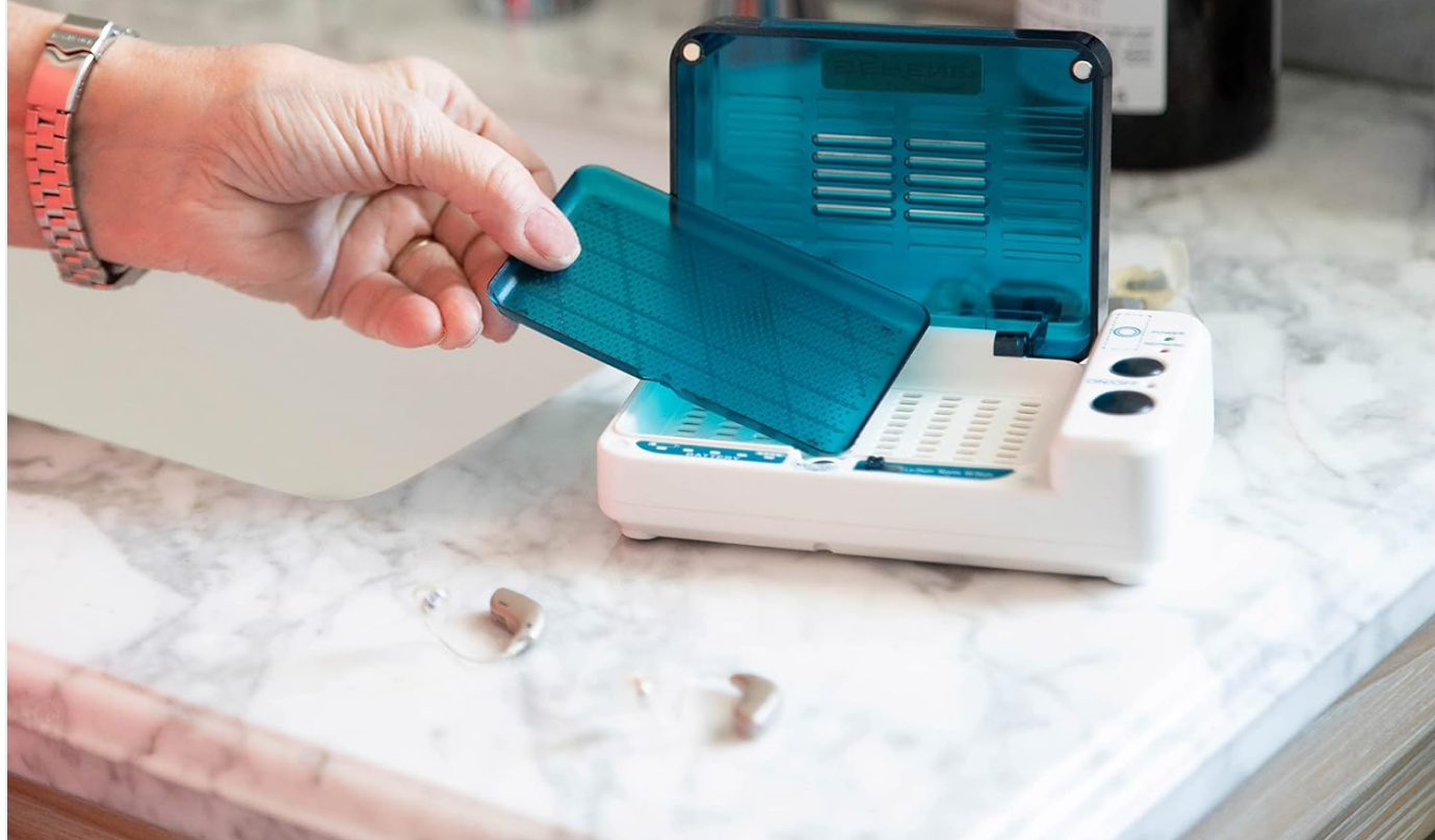
Image 6: Demonstrating the removal of the inner tray for easy cleaning.
