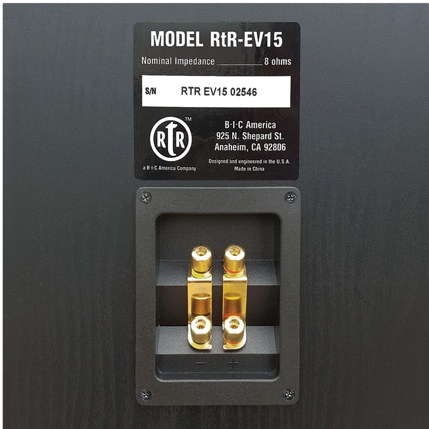
Figure 4: Rear panel connections of the BIC AMERICA RTR-EV15 speaker.
