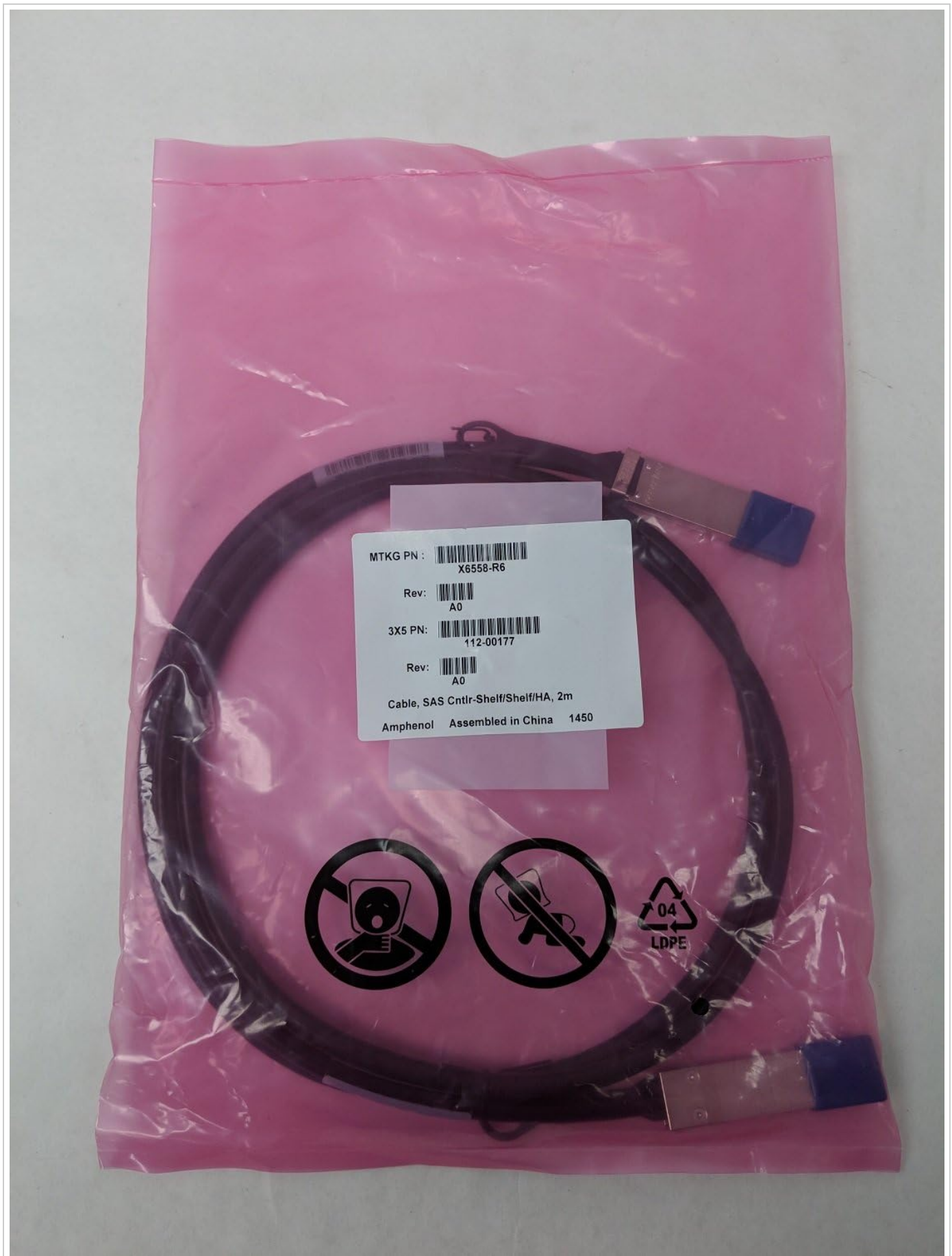
Image: The NetApp X6558-R6 SAS cable, coiled inside its sealed pink anti-static bag. A white product label is affixed to the bag, displaying the model number X6558-R6, revision A0, and indicating it is a "Cable, SAS Cntrl-Shelf/Shelf/HA, 2m" manufactured by Amphenol and assembled in China. The cable features QSFP connectors on both ends.
