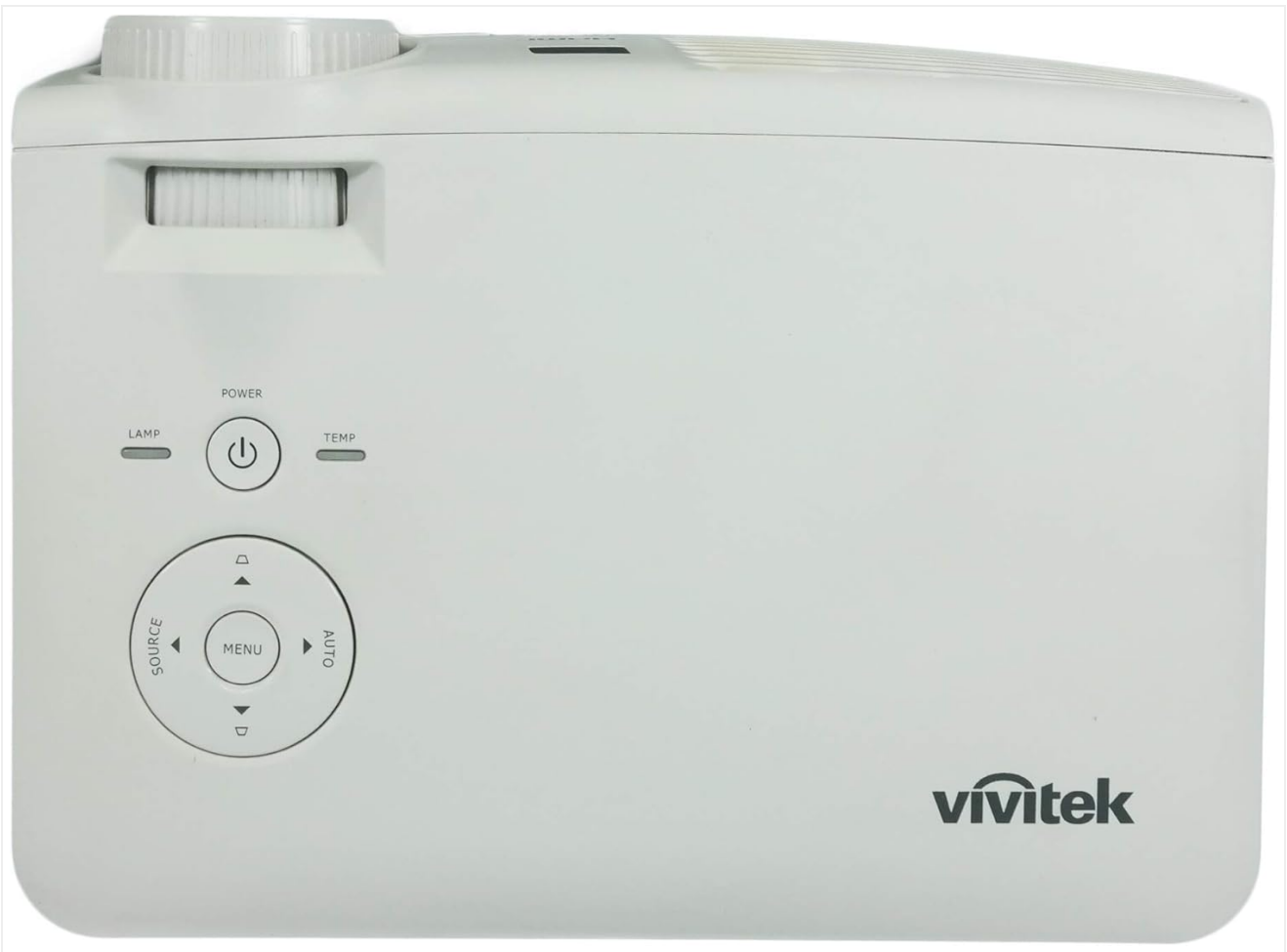
Image 3.3: Top panel of the Vivitek D511 projector, showing the control buttons and indicator lights.
