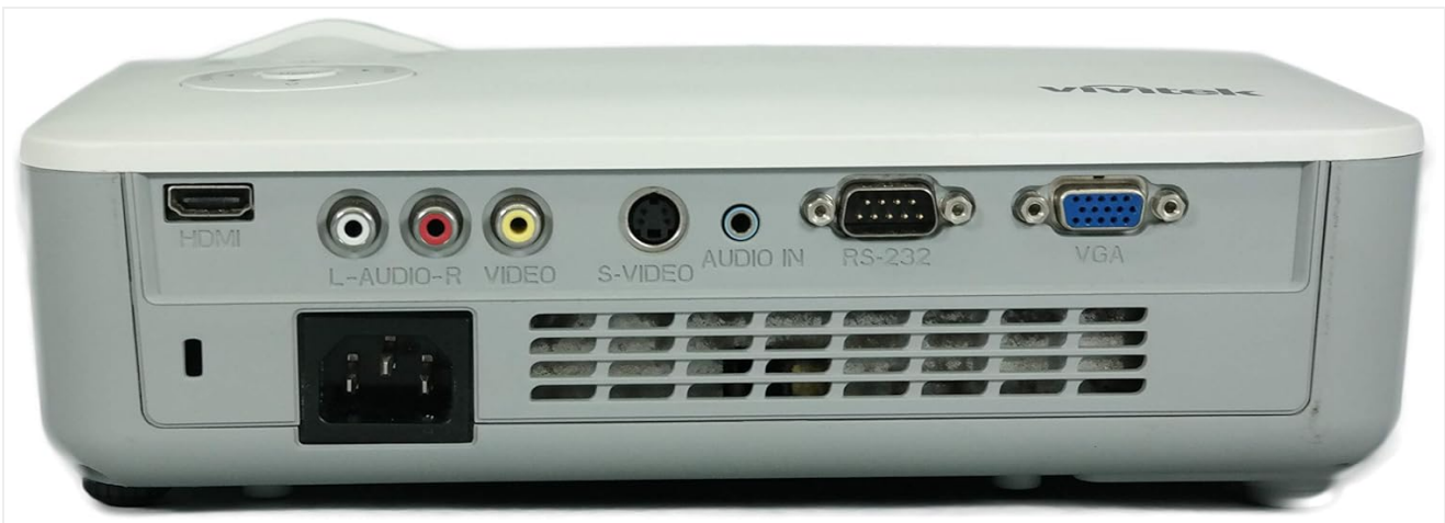
Image 3.2: Rear panel of the Vivitek D511 projector, displaying various input and output ports.
