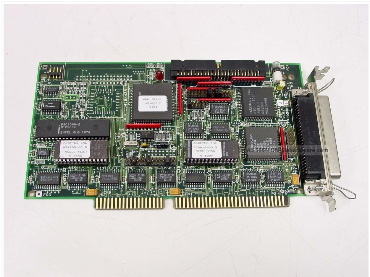
Figure 2.2: Top-down view of the Adaptec AHA-1540B circuit board, displaying the various integrated circuits, jumpers, and
