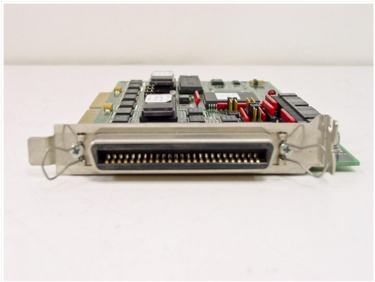
Figure 2.1: Side view of the Adaptec AHA-1540B controller, highlighting the external 50-pin SCSI connector and the ISA bus interface.
