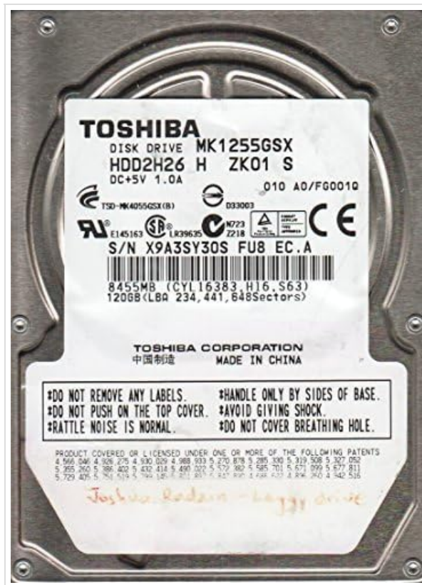
Image: Toshiba MK1255GSX 120GB Internal Hard Disk Drive. This image displays the top surface of the hard drive, featuring the product label with essential information such as the model number (MK1255GSX), serial number, power requirements (DC+5V 1.0A), and various safety and handling instructions. The label also indicates the drive's capacity as 120GB.
