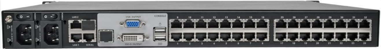
Figure 3.1: Rear view of the KVM Switch, highlighting the dual power inputs, LAN ports, console connections (VGA/DVI), and 32 RJ45 KVM ports for server connections.
