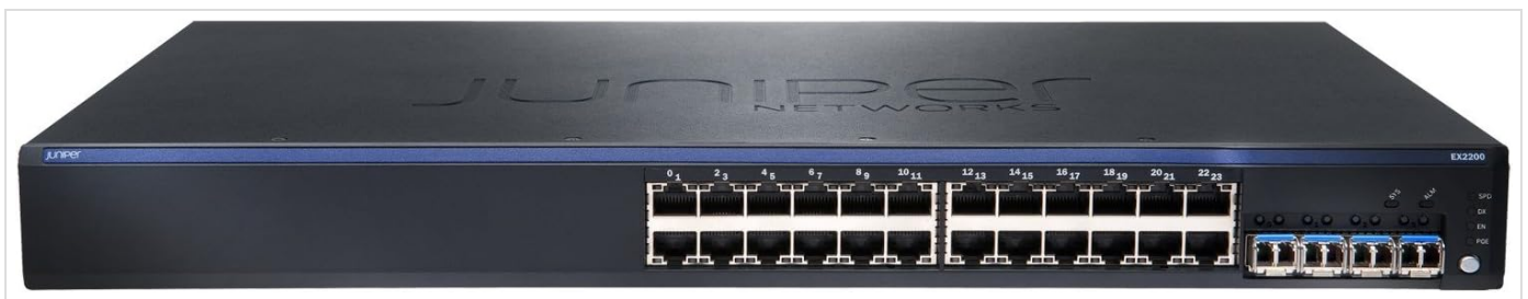
Figure 1: Front panel of the Juniper EX2200-24T-4G switch. This image displays the front panel of the Juniper EX2200-24T-4G switch. It features 24 RJ45 Gigabit Ethernet ports, numbered 0 through 23, arranged in two rows. To the right, there are four SFP (Small Form-Factor Pluggable) uplink ports, typically used for fiber optic connections. Status LEDs for system (SYS), alarm (ALM), speed (SPD), duplex (DX), enable (EN), and Power over Ethernet (POE) are also visible on the right side. Note that this specific model (EX2200-24T-4G) does not support PoE.
