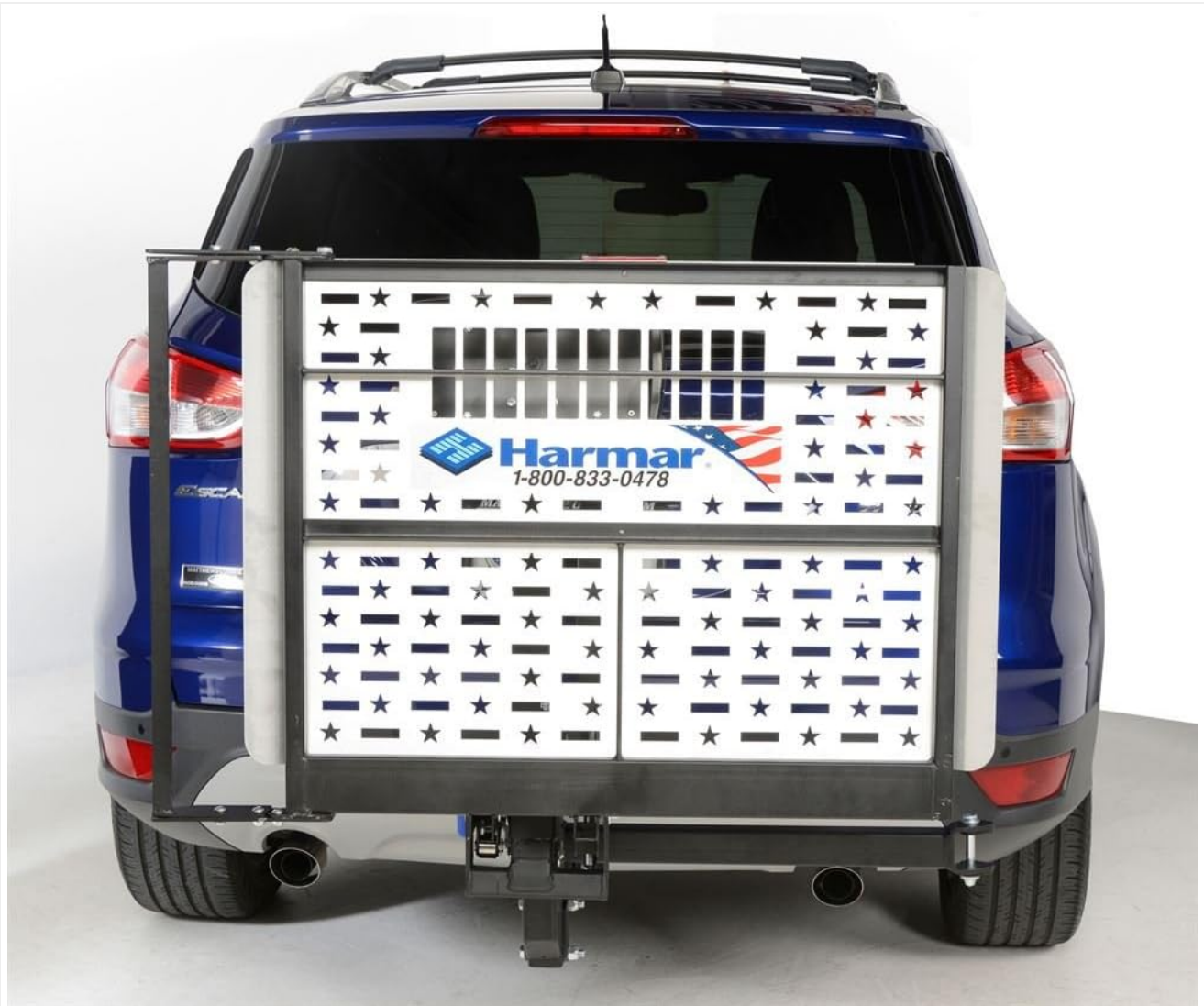
Image 2: The Harmar AL100 lift in its folded, stowed position against the rear of an SUV. This demonstrates the compact storage when not in use.
