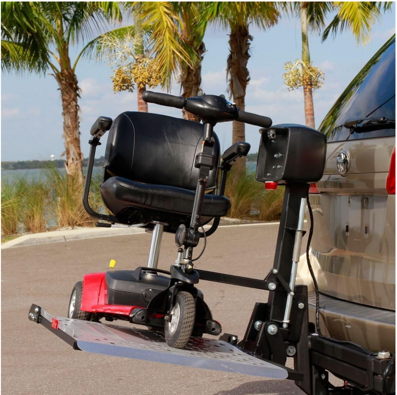
Image 4: A mobility scooter fully loaded and secured on the Harmar AL100 lift, with the platform raised and the clamping arm engaged.
