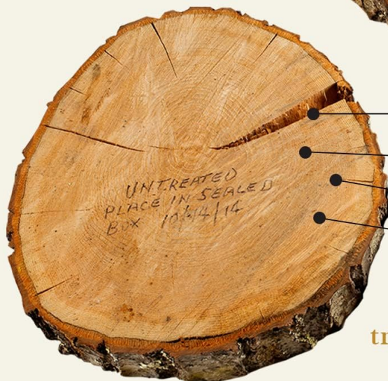
Figure 6.1: Visual comparison of Pentacryl-treated versus untreated wood after drying.
