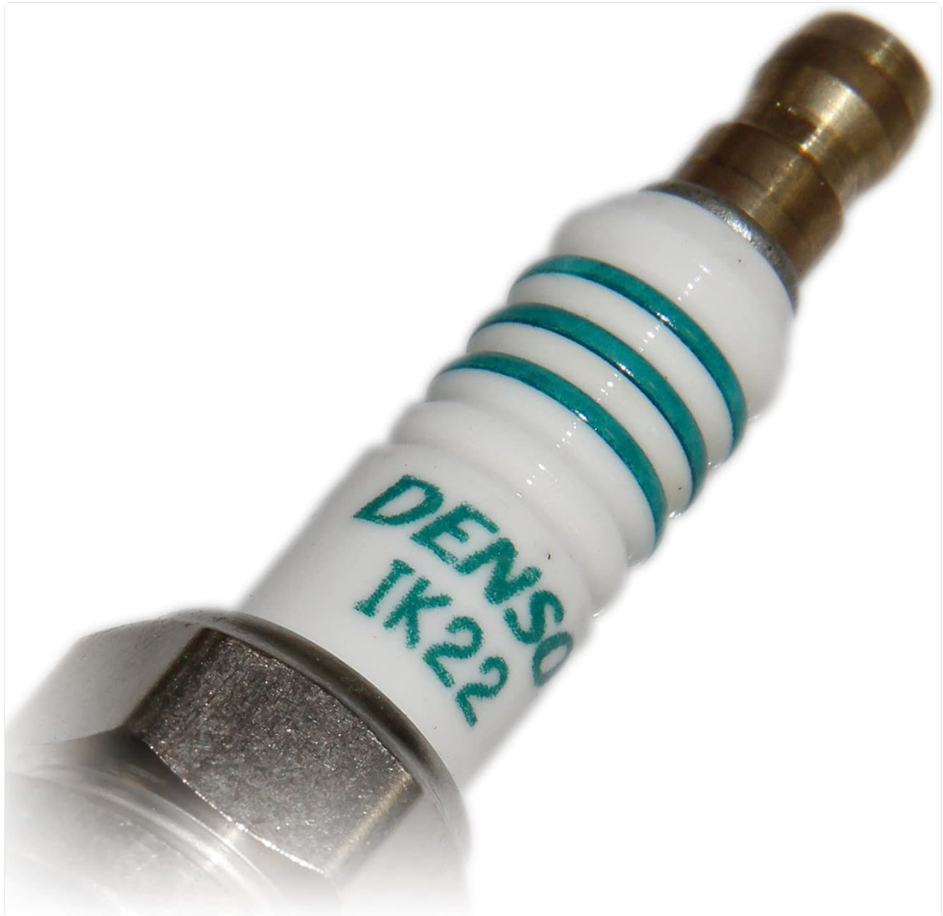
Figure 6.1: The Denso IK22 model designation clearly visible on the spark plug's ceramic insulator.
