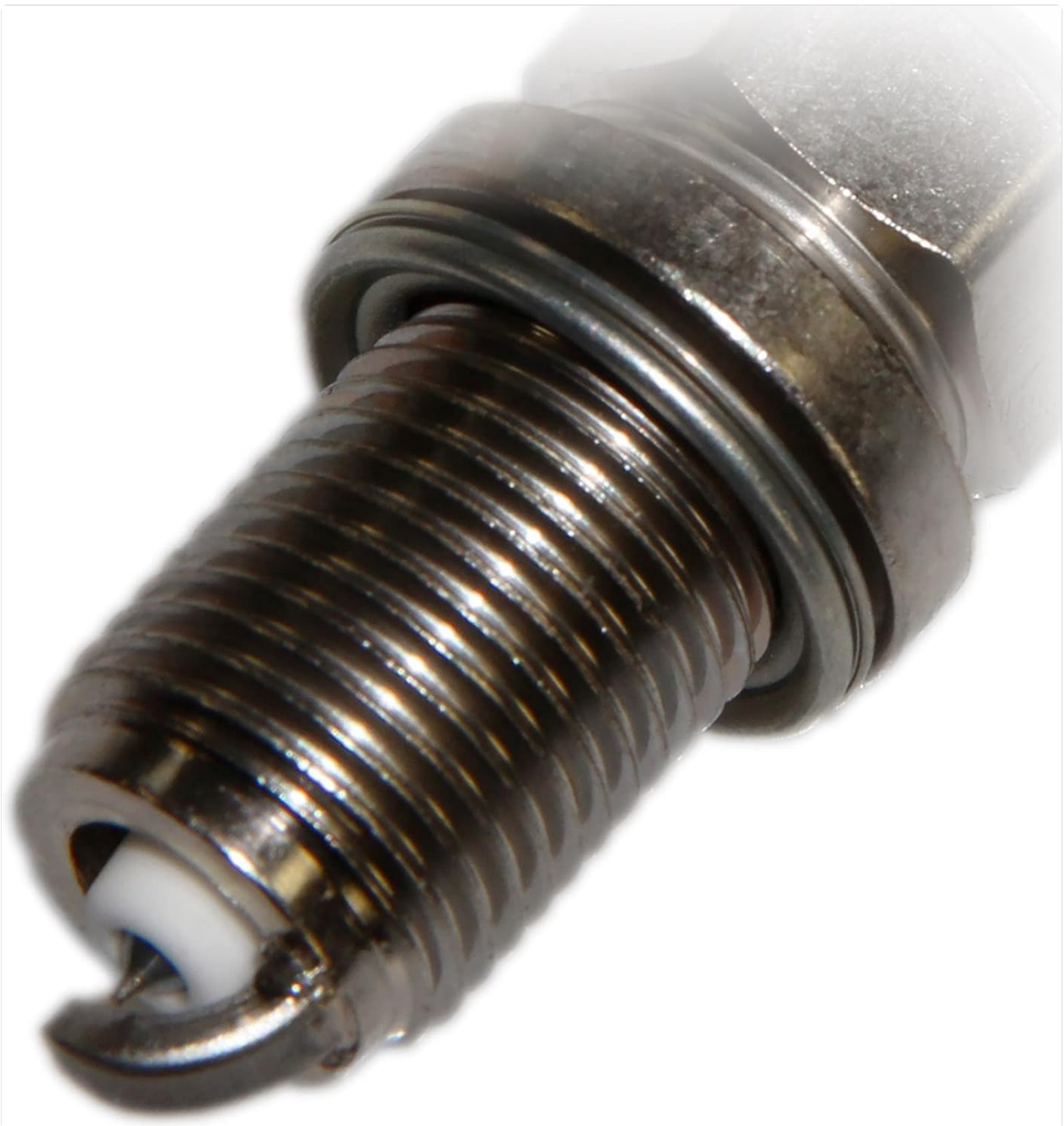
Figure 4.1: Close-up of the iridium center electrode and U-Groove ground electrode, critical for spark performance.
