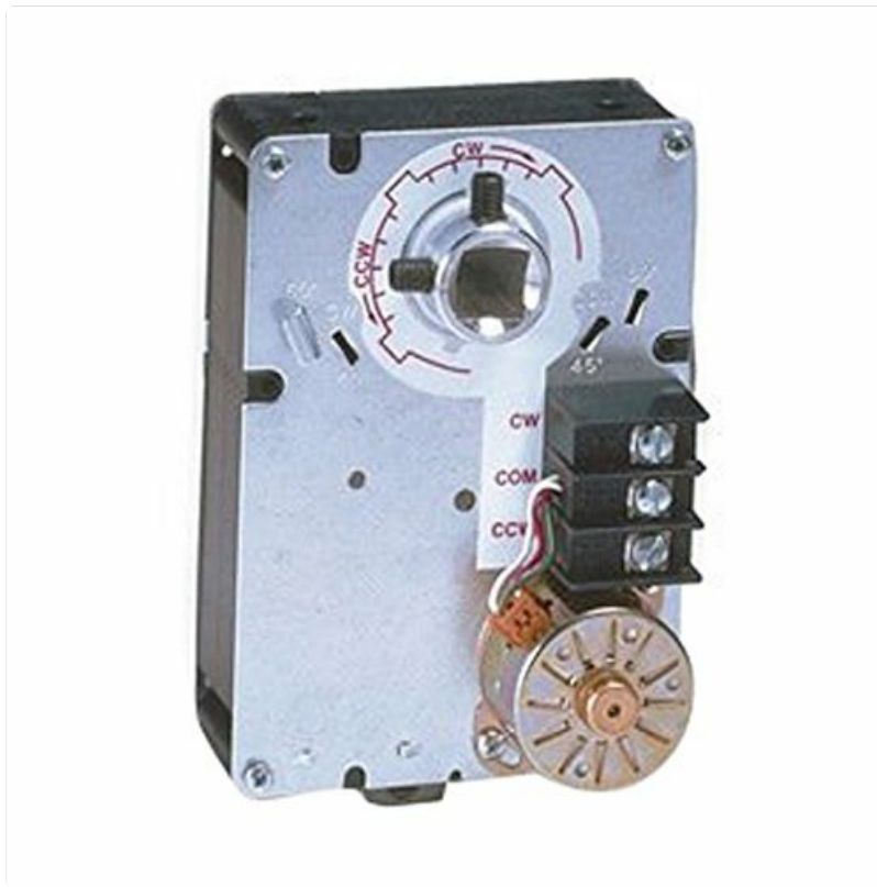
Image: Honeywell ML6161B2024 Direct Coupled Damper Actuator. This image shows the front face of the actuator, highlighting the shaft coupling mechanism at the center, the terminal block for electrical connections (CW, COM, CCV) on the right, and the internal motor assembly at the bottom right. The dial around the shaft indicates clockwise (CW) and counter-clockwise (CCW) rotation.
