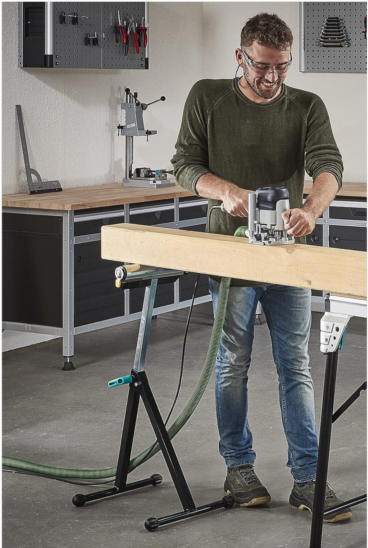
Figure 3: Supporting a workpiece during routing.
