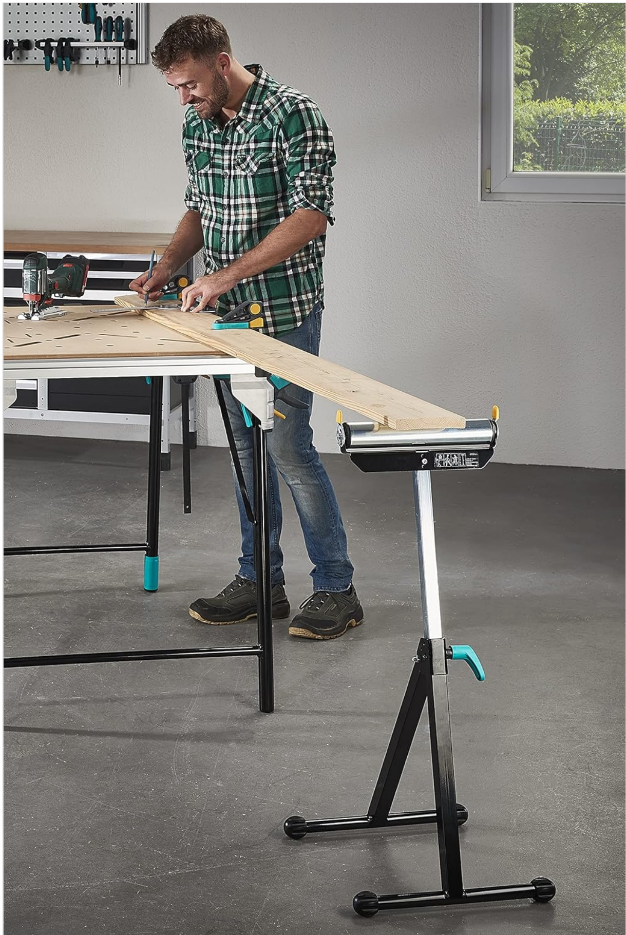
Figure 2: Trestle in use, supporting a long workpiece.
