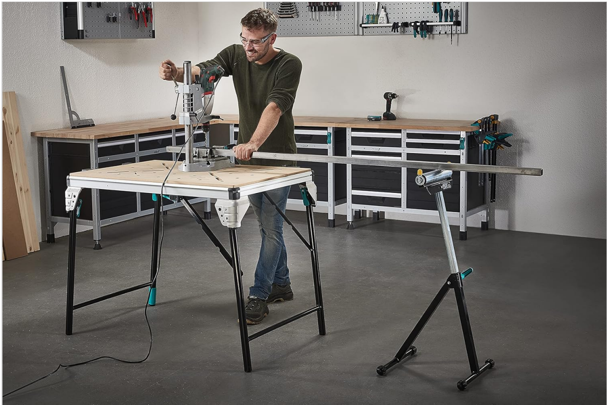
Figure 4: Supporting a metal bar during drilling.
