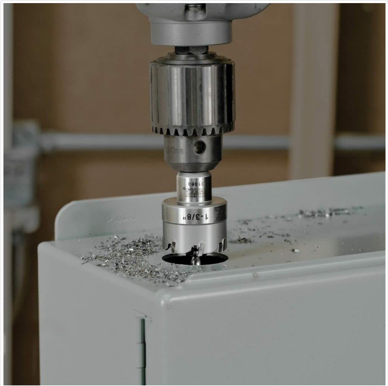
Image: A Klein Tools hole saw actively cutting a precise circular hole in a metal surface, with metal shavings visible around the cutting area.
