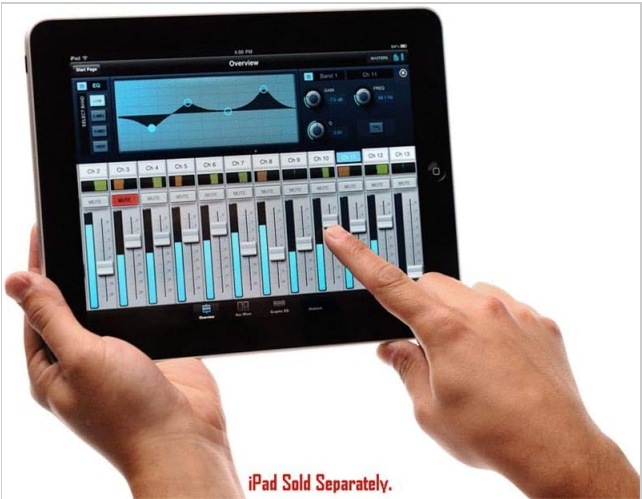
Figure 3.6.1: An iPad displaying the VSL software interface, demonstrating remote control capabilities for the PreSonus StudioLive mixer. The iPad is shown being held by two hands, interacting with the virtual faders and controls.
