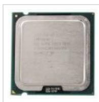
Figure 1: Intel Pentium D 915 Dual-Core CPU. This image displays the top view of the processor, showing the Intel logo and model number, with the heat spreader visible.
