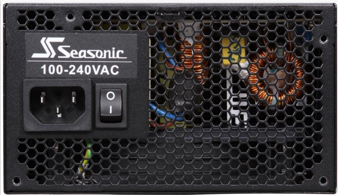
Image 4.1: Rear panel of the power supply showing the AC input and power switch.
