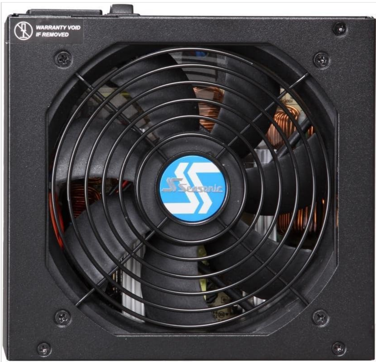
Image 5.1: Top view of the power supply, highlighting the 120mm cooling fan.
