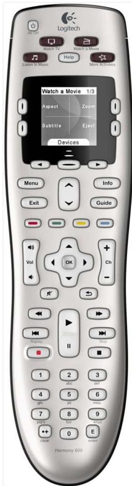
Figure 1: Front view of the Logitech Harmony 600 Universal Remote. This image displays the remote's full layout, including the LCD screen, activity buttons, navigation controls, and numeric keypad, highlighting its ergonomic shape and button arrangement.
