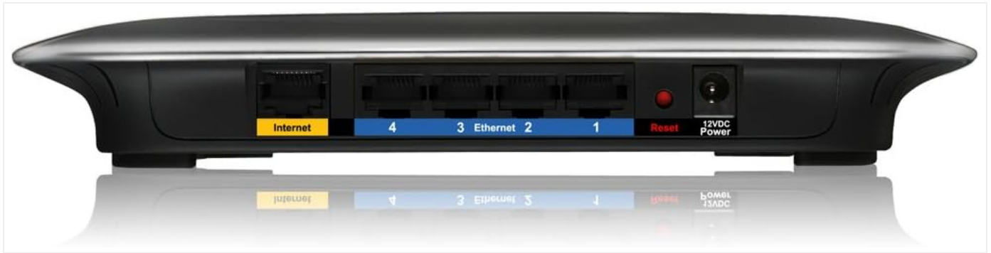
Figure 2: Rear panel of the Linksys E2000 router, highlighting the Internet (WAN) port, four Gigabit Ethernet (LAN) ports, power input, and reset button.
