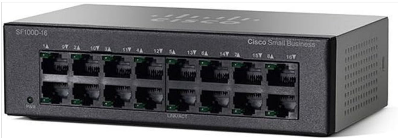
Figure 4.2: Rear view of the Cisco SF100D-16 switch, displaying the 16 Fast Ethernet ports and power input.
