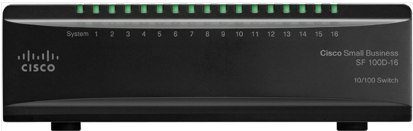
Figure 4.1: Front view of the Cisco SF100D-16 switch, showing the System LED and 16 port status indicators.
