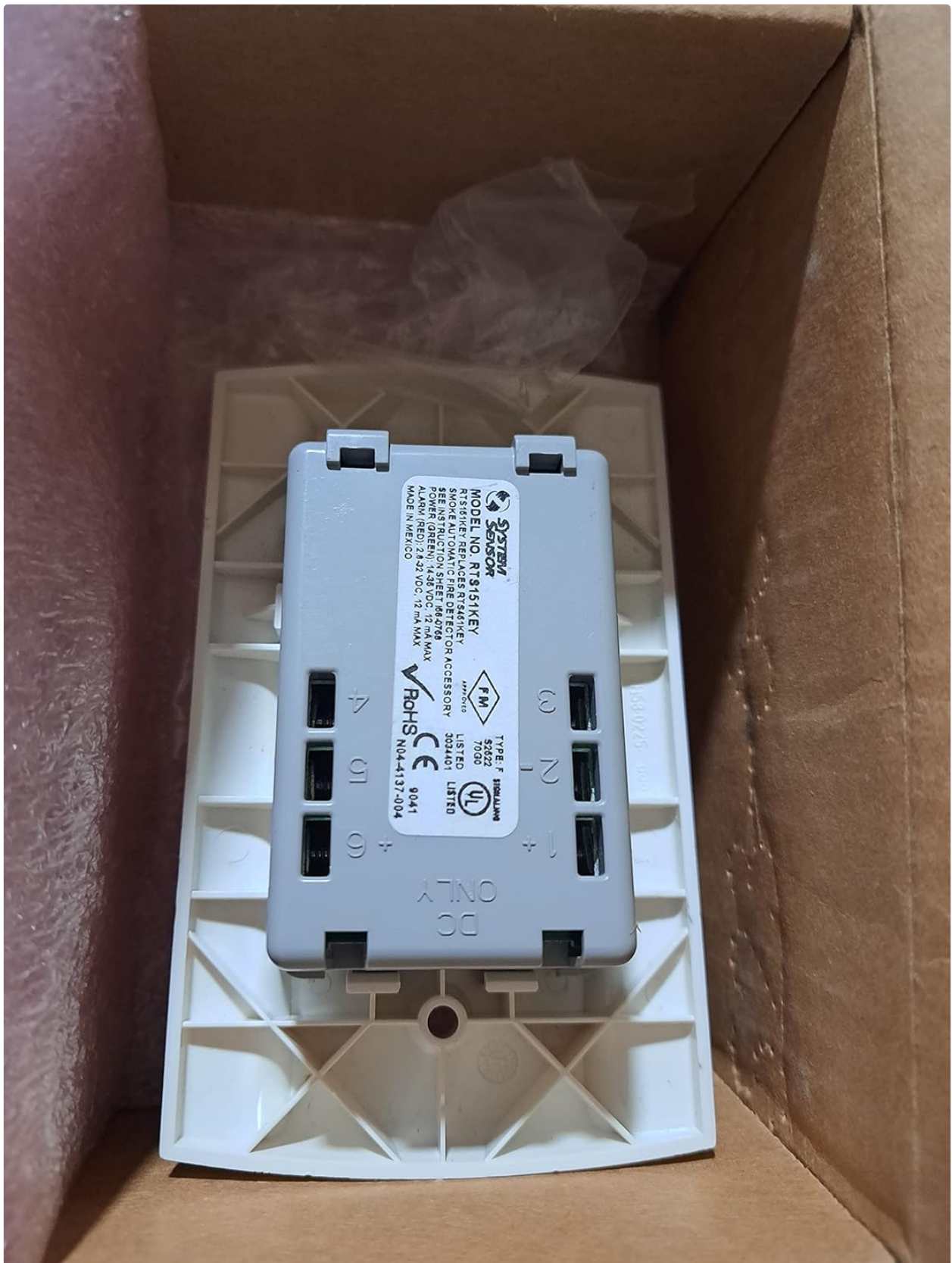
Figure 4.1: Rear view of the RTS151KEY, showing terminal block connections for wiring.
