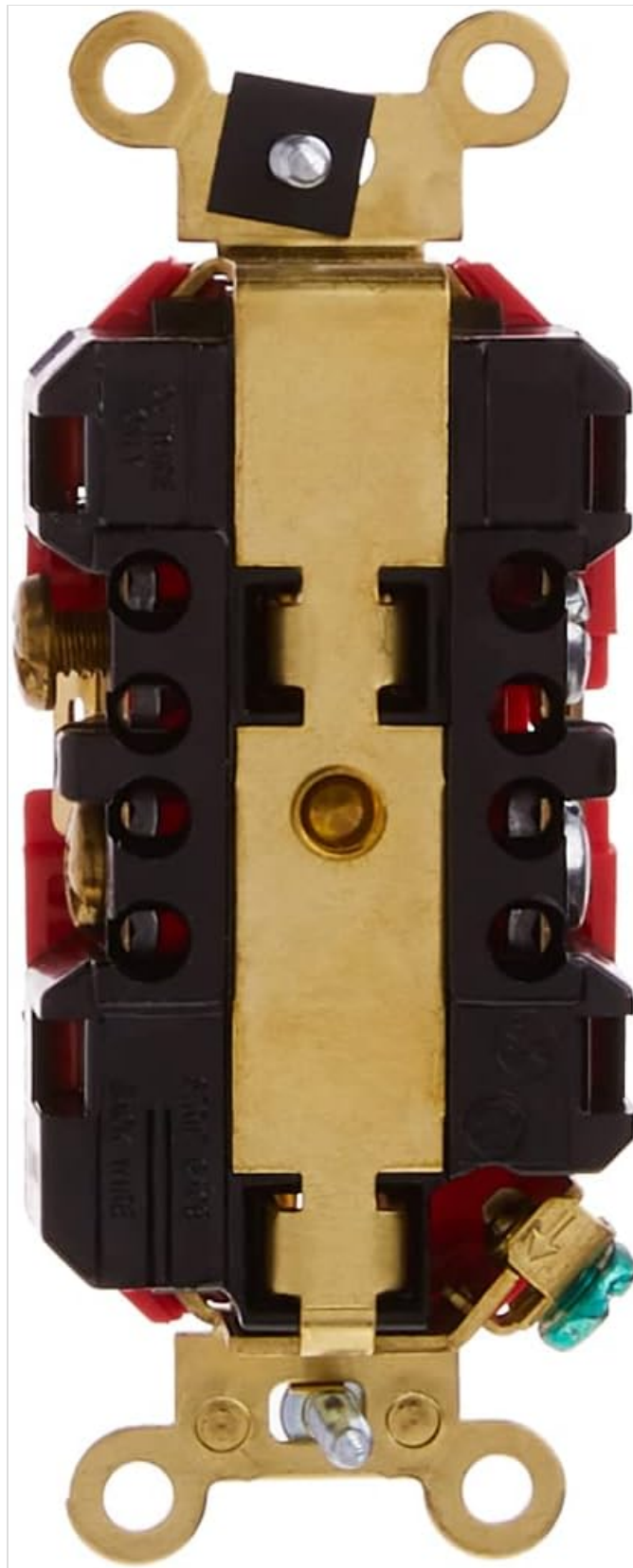
Figure 3: Back view of the Leviton 5362-R receptacle. This image provides a clear view of the wiring terminals, including the brass-colored hot terminals, silver-colored neutral terminals, and the green grounding screw. The sturdy construction of the device is evident.
