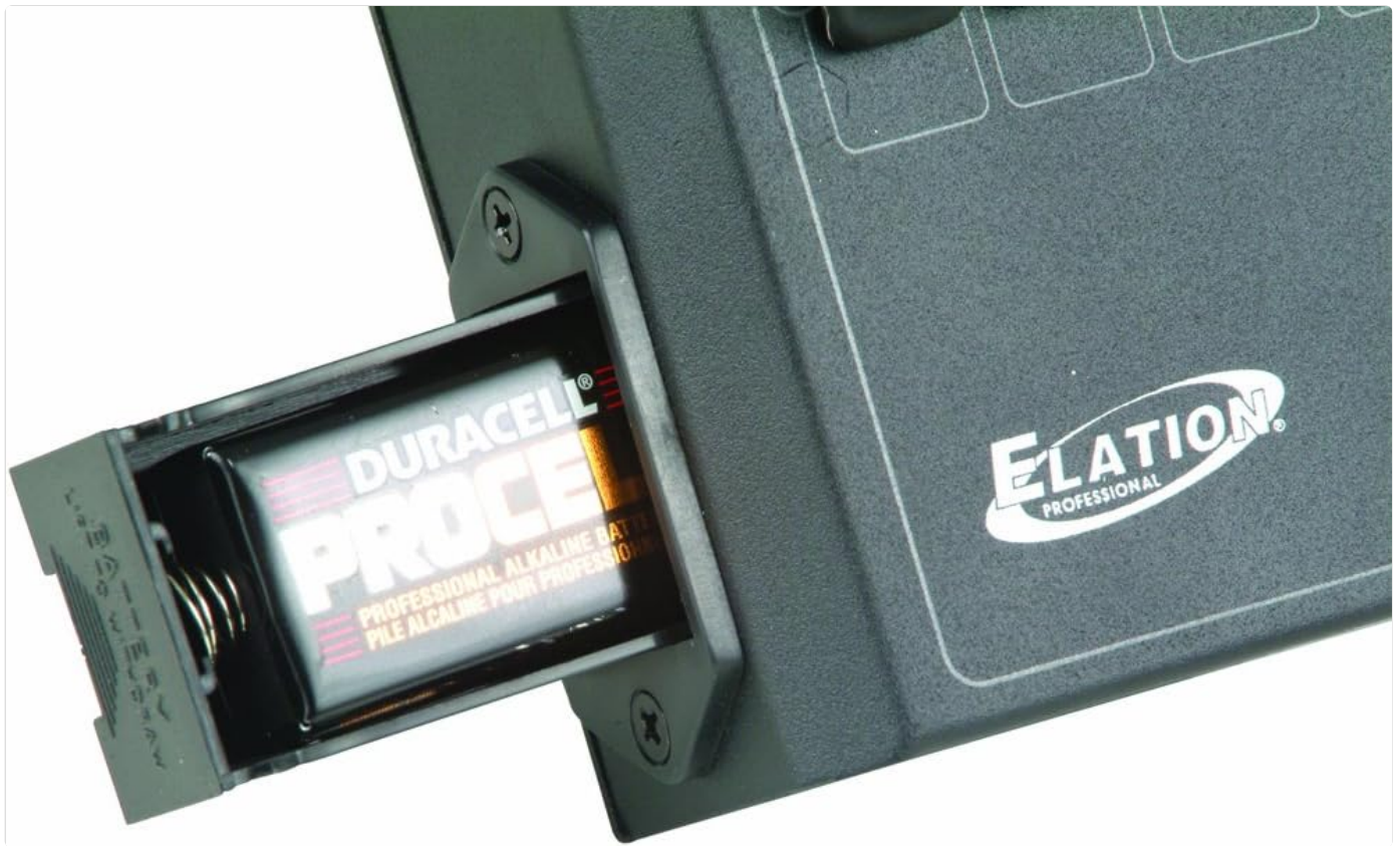
Figure 4.2: Side view of the Elation SDC-6 v2 DMX Controller, illustrating the battery compartment for optional portable power (battery not included for primary operation).
