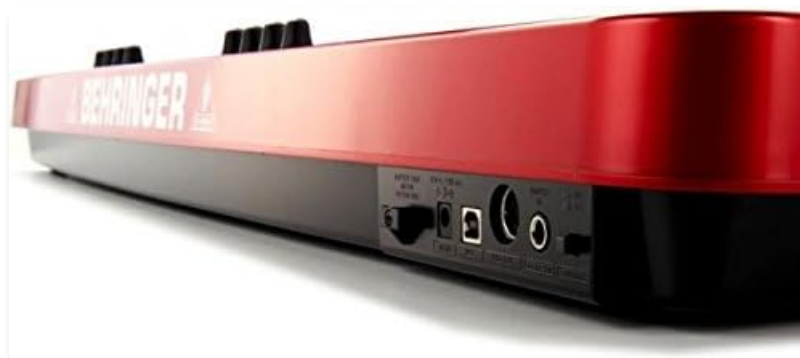
Figure 2: Rear panel connections of the UMX610, including USB, MIDI Out, and audio ports.
