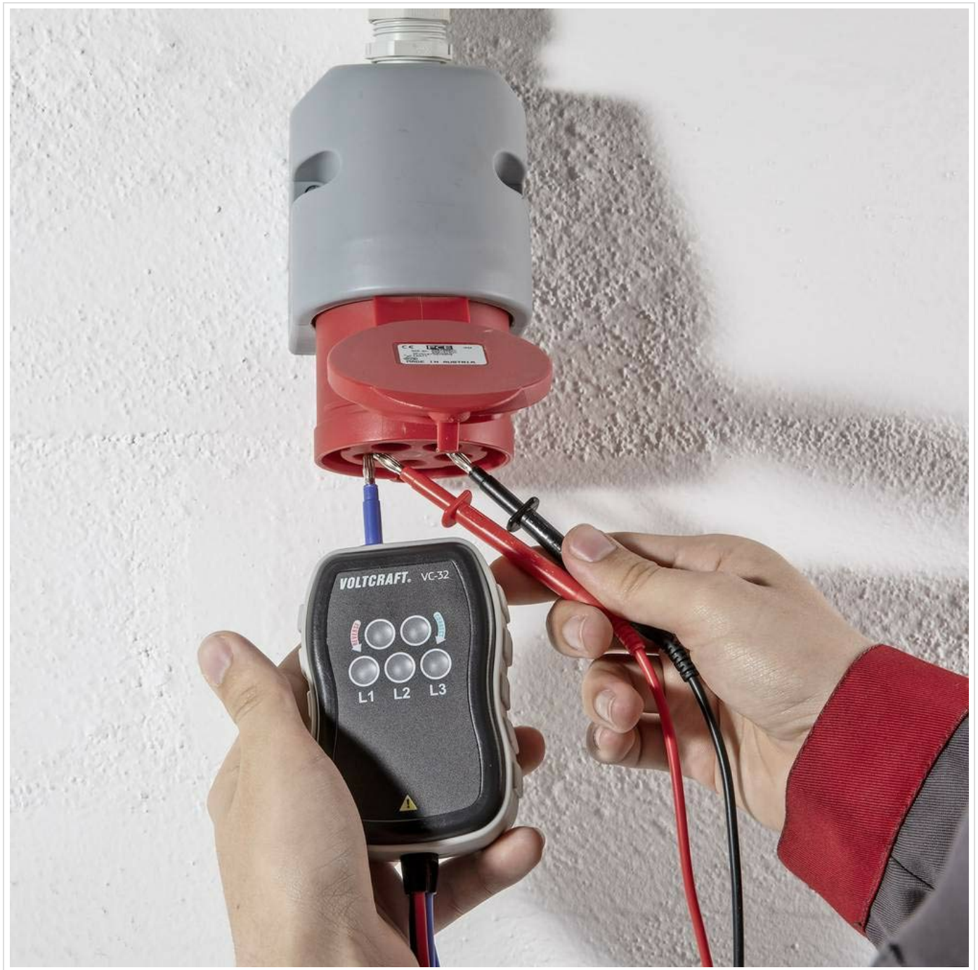
Figure 5.1: User connecting the VC-32 to a three-phase electrical socket for testing.
