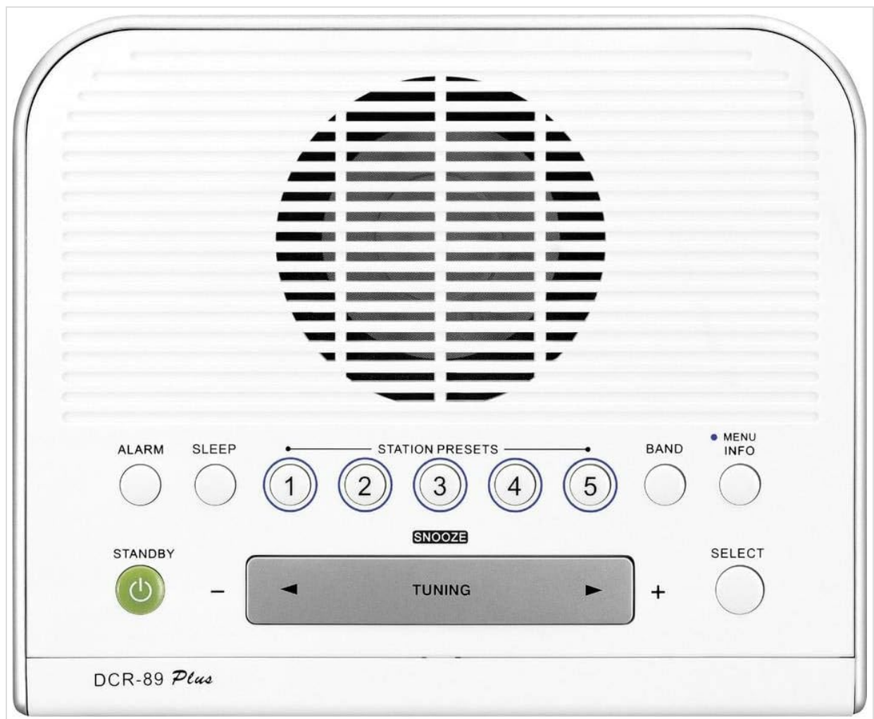
Image: Top view of the Sangean DCR-89+ radio, illustrating the speaker grille and control buttons. Buttons include ALARM, SLEEP, STATION PRESETS (1-5), BAND, MENU/INFO, STANDBY, TUNING controls, and SELECT.
