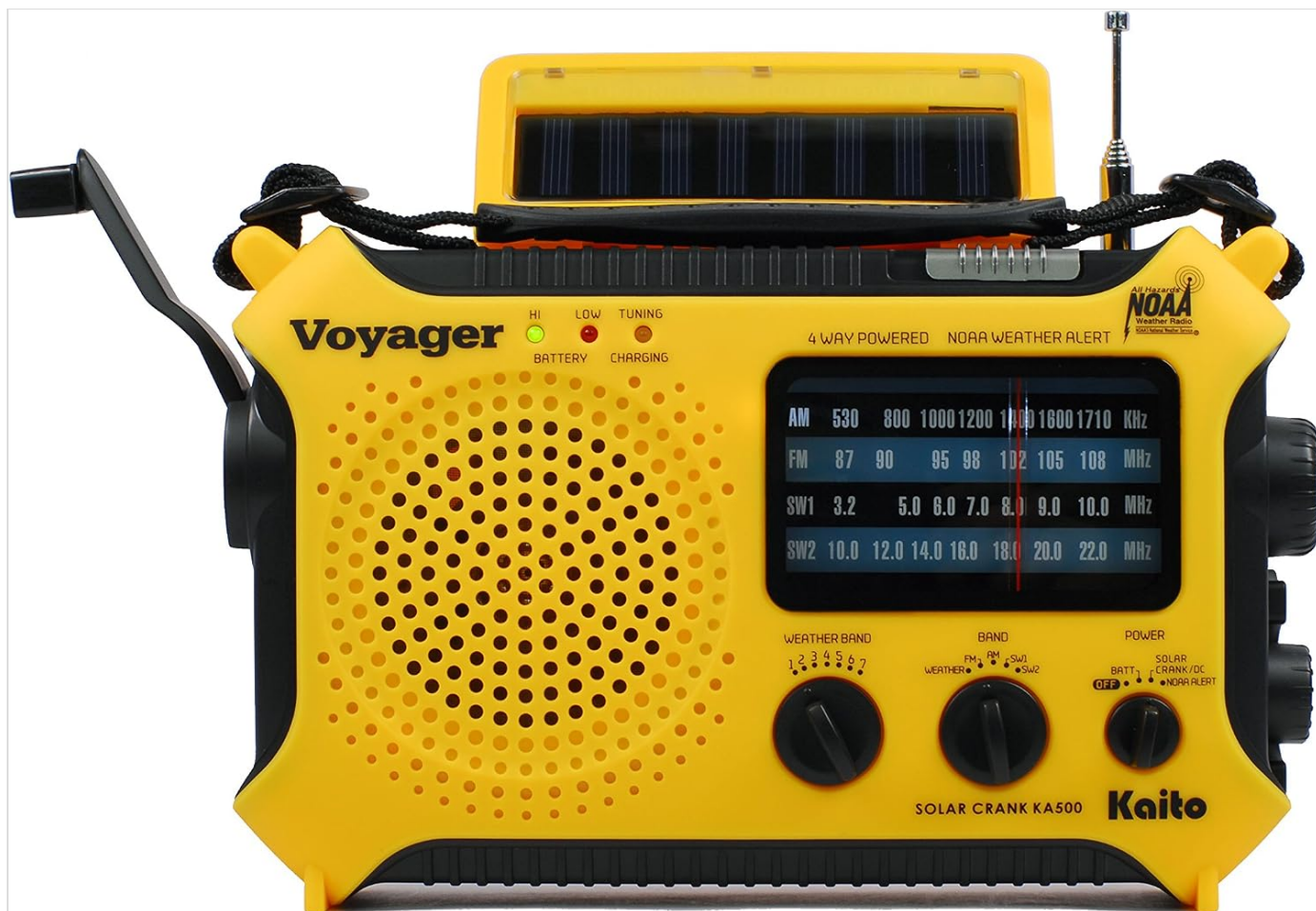
Image 4.1: Front panel of the Kaito KA500 radio, highlighting the tuning dial, band selector, and power controls.
