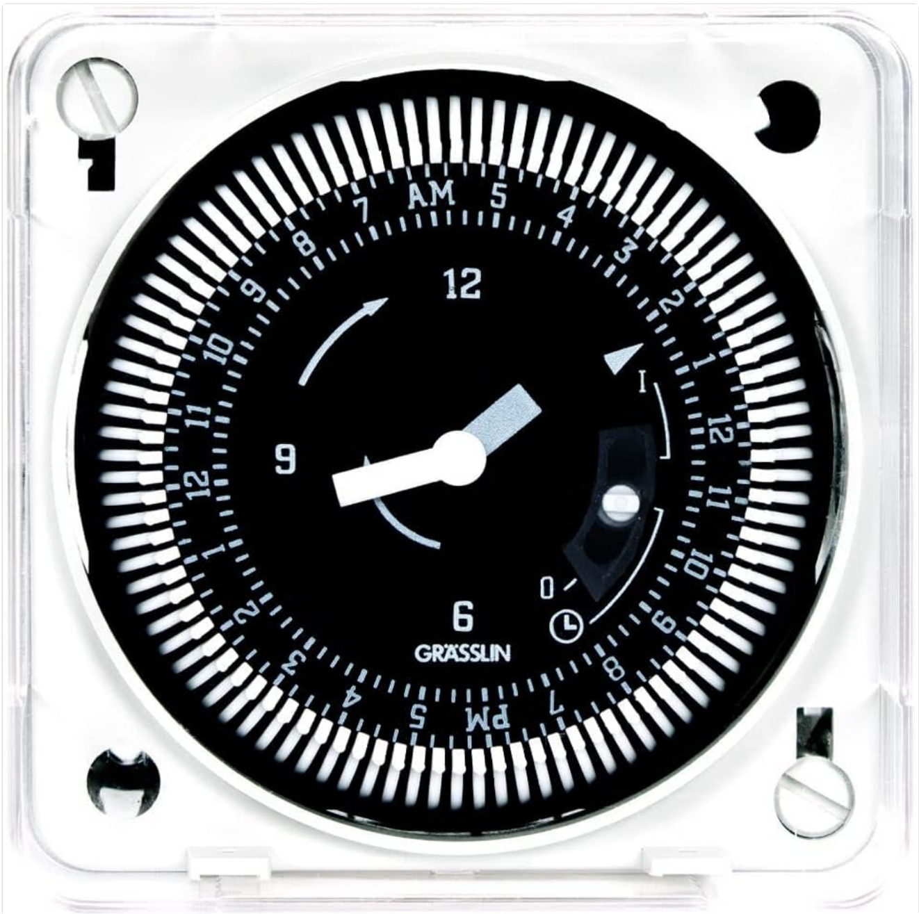
Image: Front view of the Intermatic MIL72ESTUZH-120 timer. The device features a clear protective cover over a black dial. The dial displays a 24-hour format with AM/PM indicators and minute markings. A central clock mechanism with hour and minute hands indicates the current time. The outer edge of the dial contains captive trippers for setting ON/OFF periods. A manual override switch is visible on the right side of the dial.
