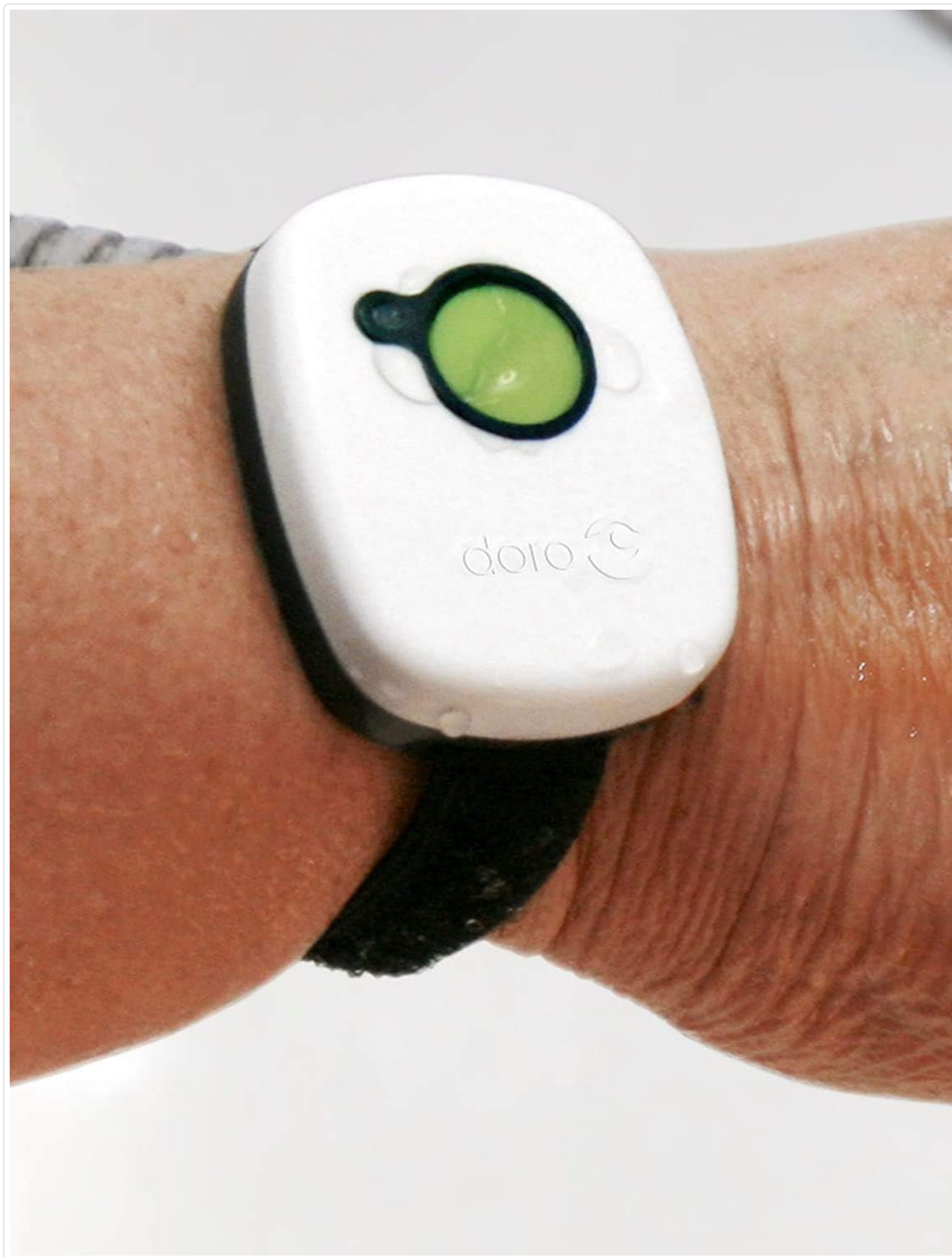
Image: A close-up view of the Doro SecurePlus 50rc medallion on a wrist, visibly wet, confirming its IP56 waterproof rating.
