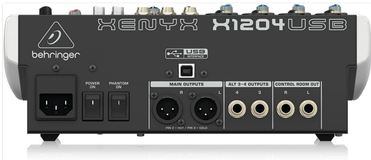
Figure 3: Rear view of the mixer, showing the power input, power switch, phantom power switch, and the USB interface port.
