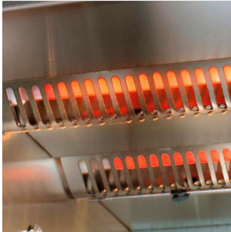
Figure 2: Close-up view of the overhead quartz heating elements inside the Equipex FC-33/1 oven, showing them glowing red during operation.
