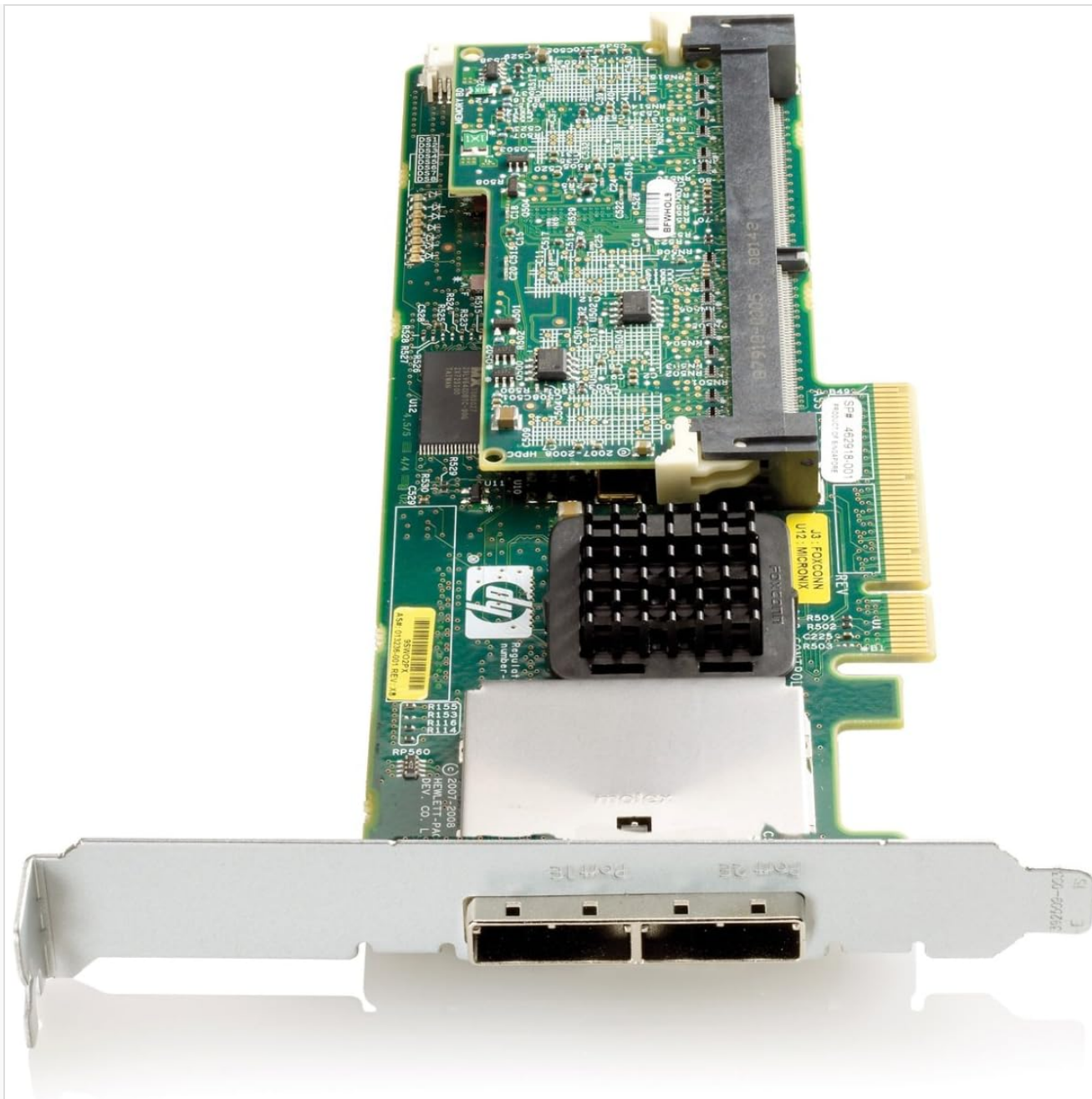
Image 1: Front view of the Hewlett Packard Smart Array P411 RAID Controller. This image displays the full-height PCI Express card with its various components, including the heatsink, SAS ports, and the PCI Express connector. The card is designed for installation into a server's expansion slot.
