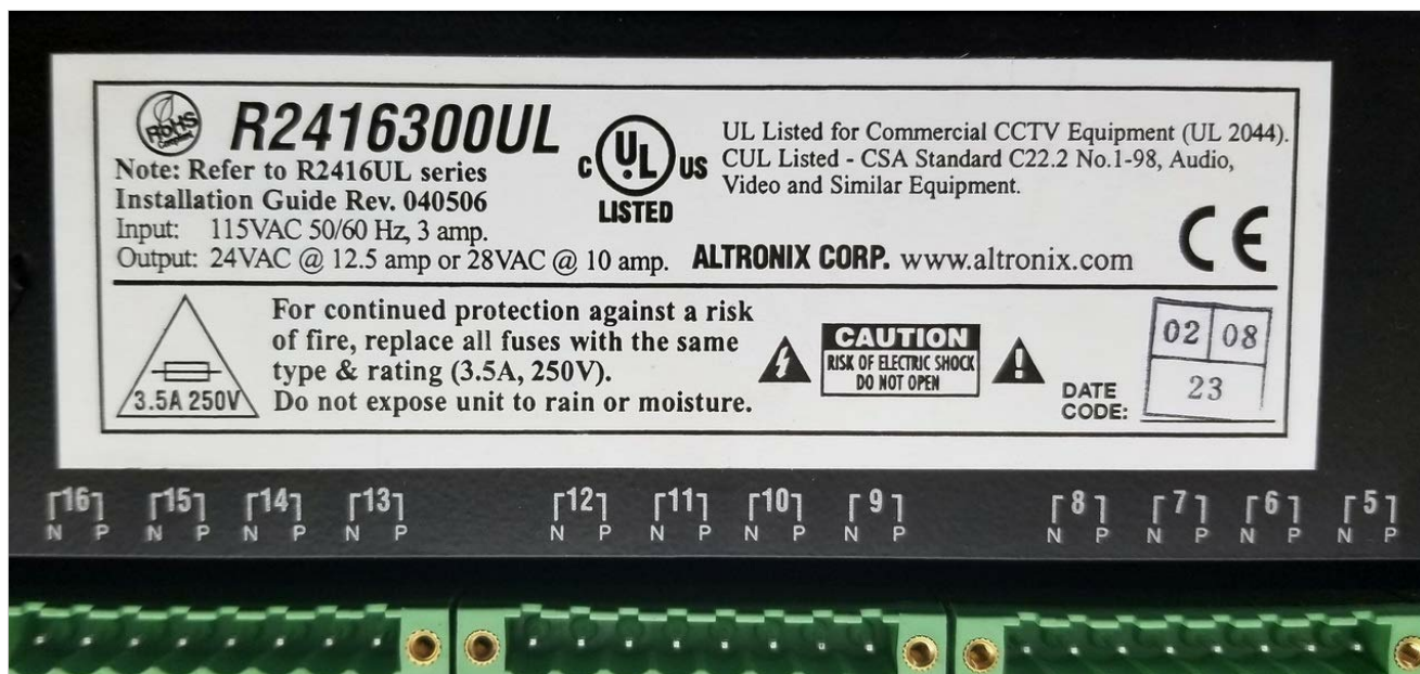
Figure 3: Close-up of the rear product label and output terminal blocks. This image provides a detailed view of the product specifications, safety warnings, and the green removable terminal blocks for connecting output devices.
