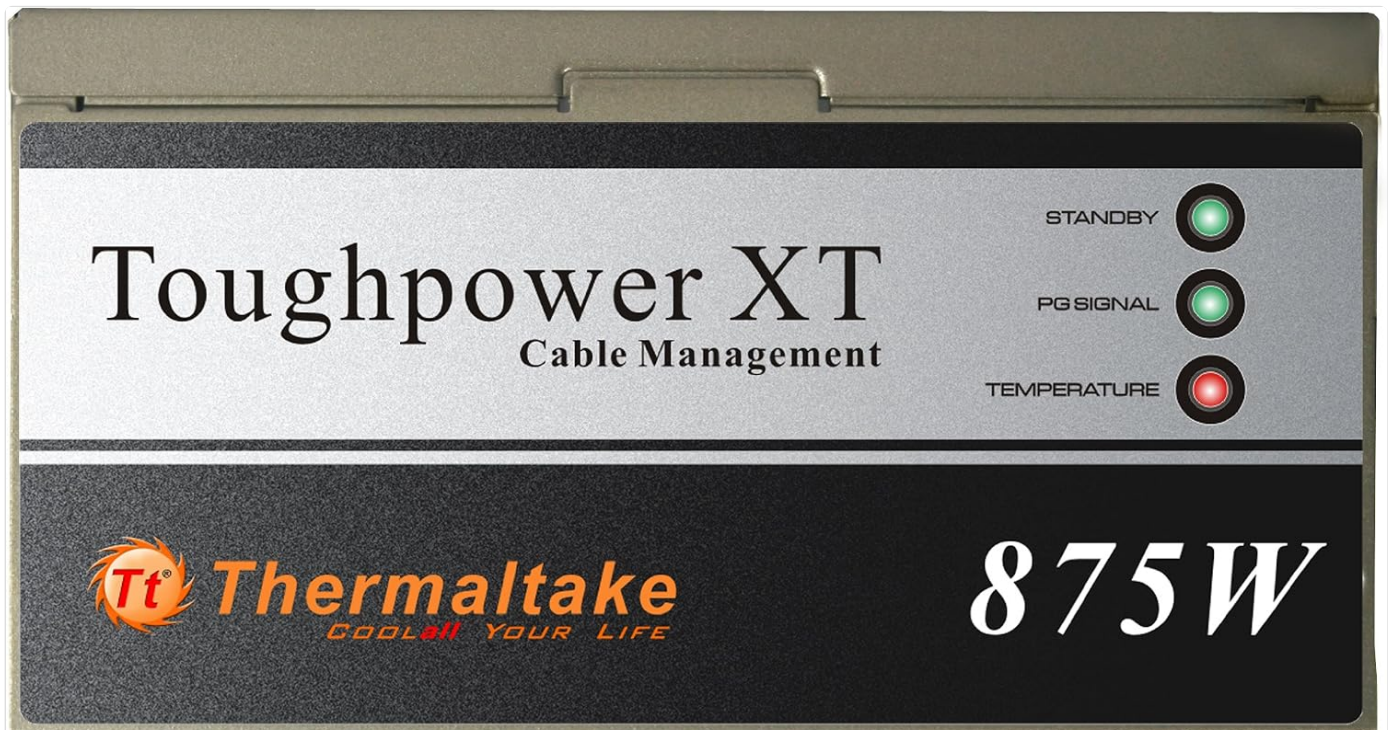
Figure 5: S.P.T. Status Indicators showing an over-temperature warning (red TEMPERATURE LED).
