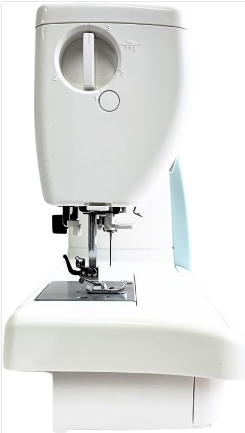
Figure 7: The thread tension dial, used to regulate the tightness of the upper thread for optimal stitch formation.
