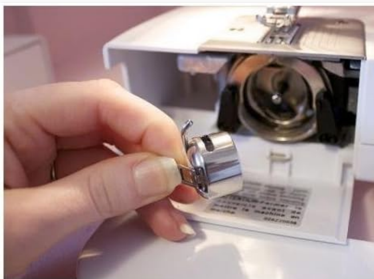
Figure 4: A hand demonstrating the removal or insertion of the bobbin case, located in the front-loading bobbin area of the machine.
