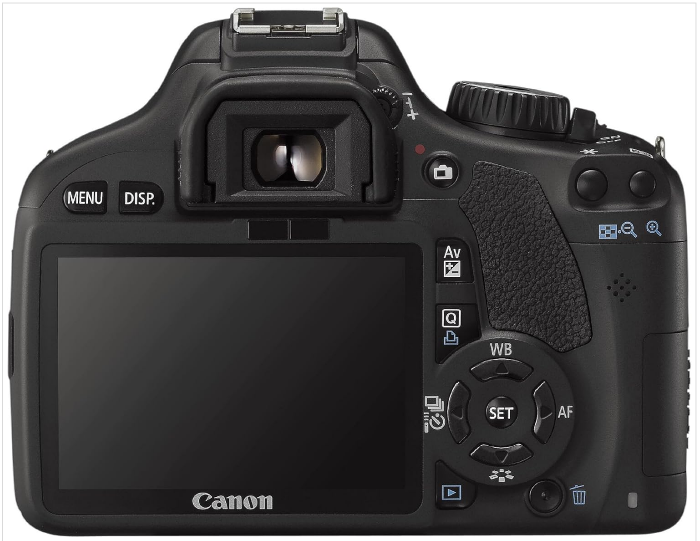
Figure 2.3: Rear view of the Canon EOS 550D, showcasing the 3.0-inch LCD screen, viewfinder, and various control buttons for menu navigation and image playback.
